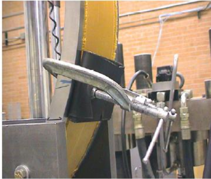
Figure 17. Kevlar® Fabric Clamped to Steel Test Ring
