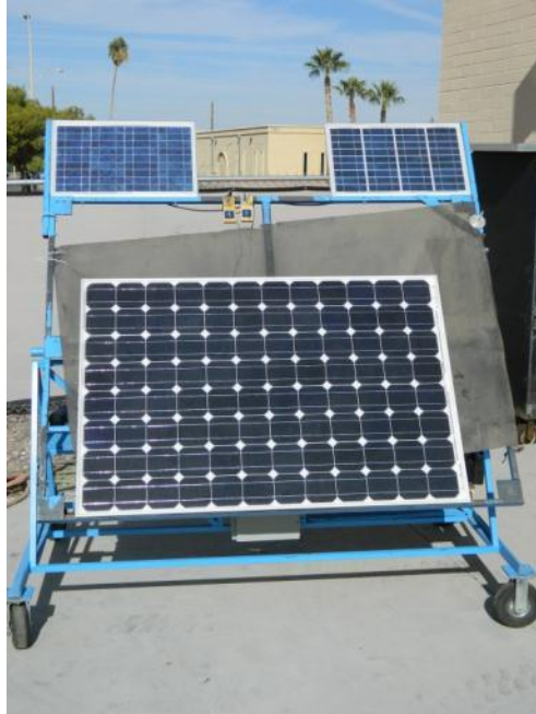
Figure 3.4: Visual inspection was performed under natural sunlight
