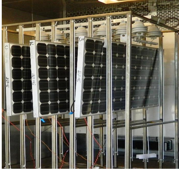
Figure 3.16: Modules hanging from ceramic insulators on a rack.
