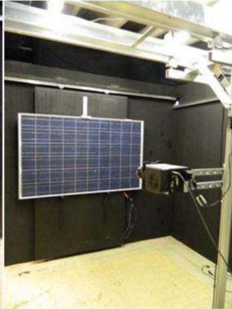
Figure 3.6: A module is shown on an adjustable rack in front of the EL camera.
