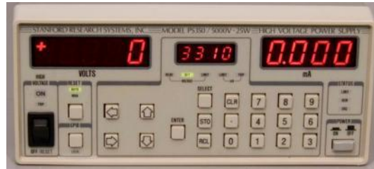
Figure 3.14: Front side control panel of the PS350 power supply.
