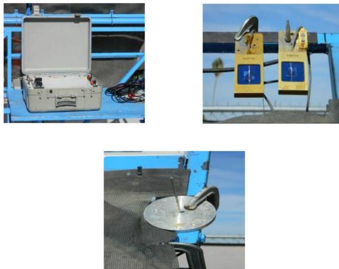
Figure 3.11: Daystar DS 100 IV curve tracer (top-left), Reference cells (top-right), Sundial (bottom).
