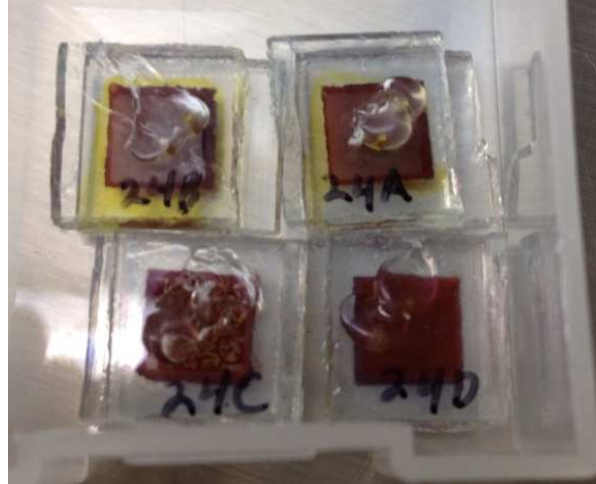
Figure 14: Effects of leakage in liquid and gel cells from the same batch
