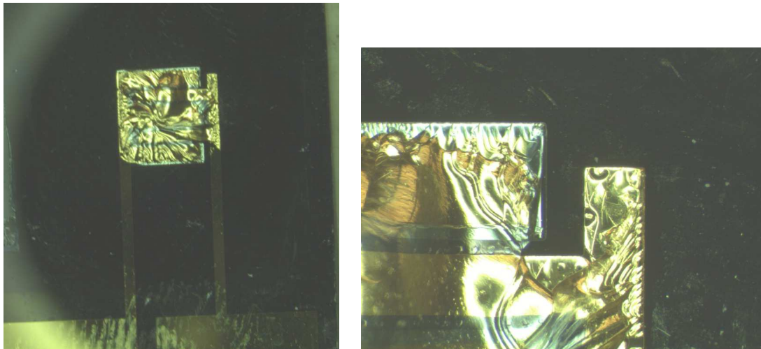
Figure 9.6: Micrograph of unsuccessful PDMS bonding onto the microfabricated IS-FET (left). Bonding only occurred on the raised areas of gold or nitride (right). The width of the gold extending pad to the sensing region where attachment occurred is 500\ \mu\text{m} .
