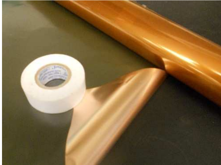
Figure 12.3: Photograph of Pyralux shown folded over to expose the copper side. Coverlay material is shown rolled next to the Pyralux and can also be cut to size.
