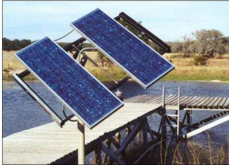
Figure 5.1: A commercial passive tracking system manufactured by Zomeworks Corporation is pictured [69]. Low boiling point fluid is contained in the tubing running along the left and right sides of the solar panels. Solar heating causes the system to track sun position.
