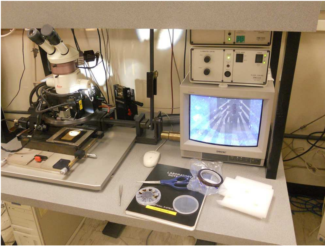
Figure 12.7: Photograph of the Finetech Picoplacer used for flip chip assembly. Assembly is done on the heated stage under the microscope, shown on the left side of the picture. A monitor, on the right, is attached to the microscope to aid in alignment. The chip and stage can be heated independently using computer control.
