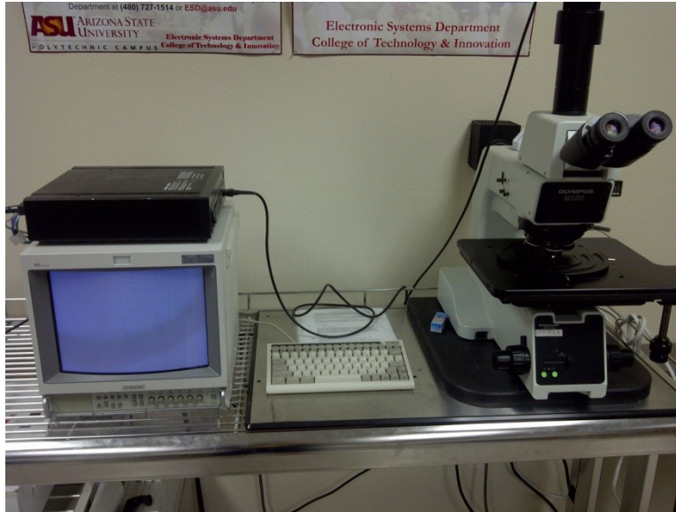
Figure 3.5: Microscope and monitor used to view TiO 2 defects
