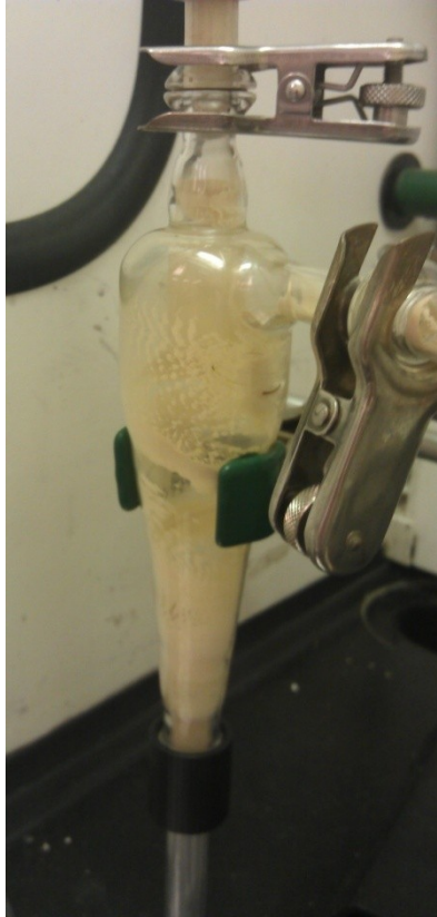
Figure 3.3: Cyclone used for powder collection in the spray dryer, containing \text{CeO}_2 .
