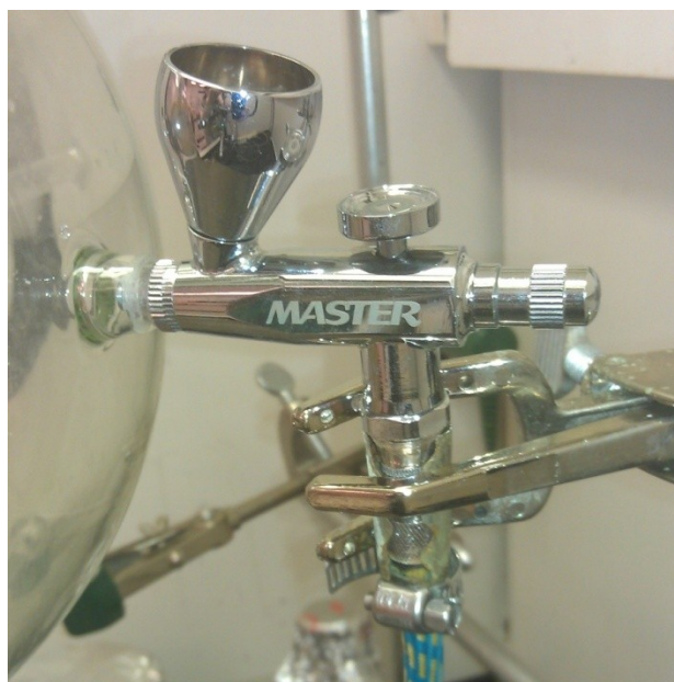
Figure 3.1: Air brush used in spray drying system to atomize precursor solution.
