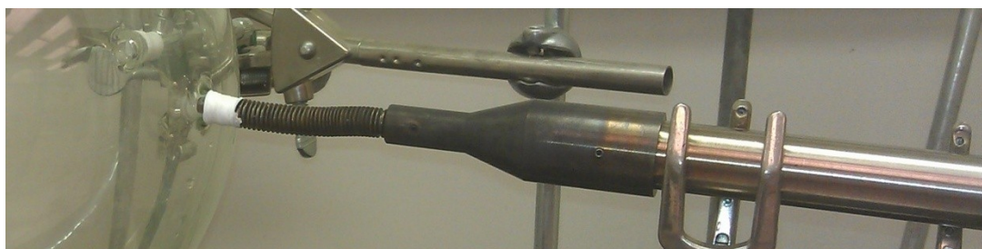
Figure 3.2: Heat gun providing hot air for drying, attached to the drying chamber of the spray dryer.
