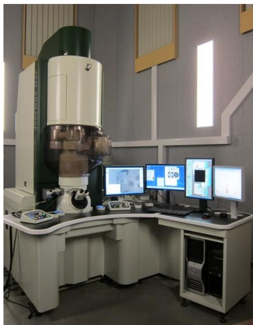
Figure 2.12: JEOL ARM 200F transmission electron microscope at Arizona State University.
