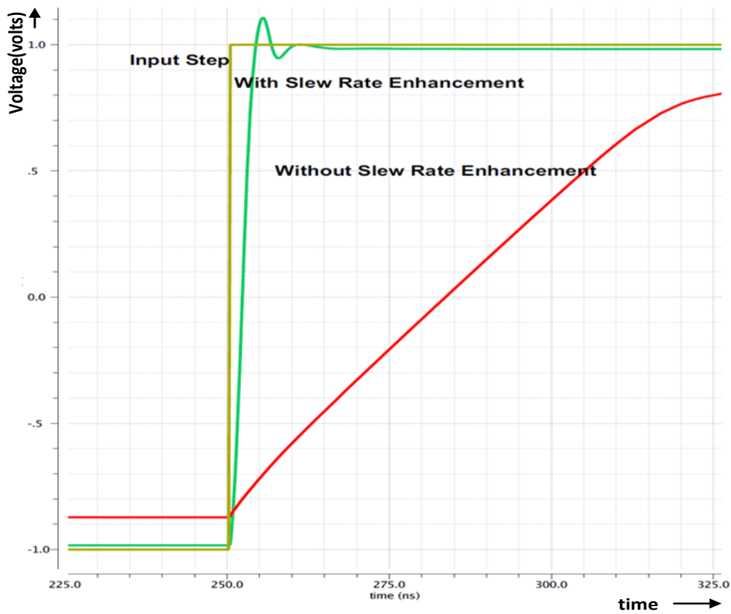
Figure 5-9 Step response of estimation amplifier with and without slew rate enhancement
