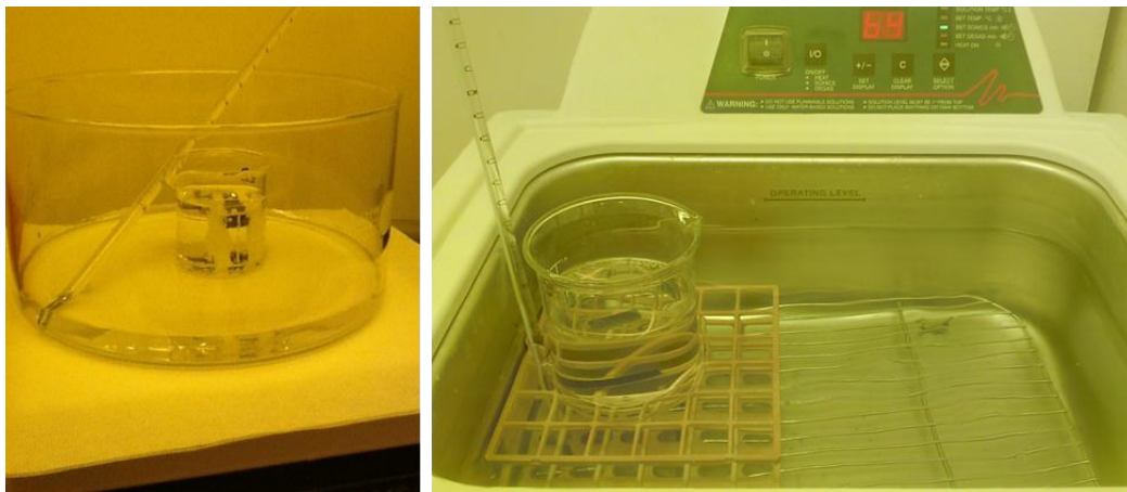
Figure 11: KOH etching experimental setup. Left panel: Hotplate, with magnetic stirring. Right panel: Heated ultrasonic bath.
