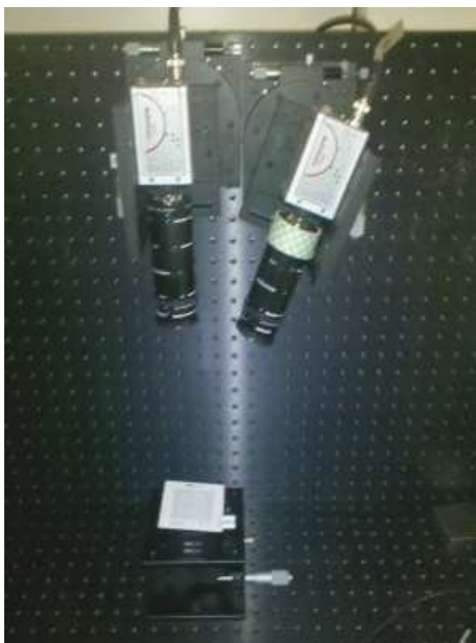
Figure 4.1: Optical breadboard setup for calibration with the two 8 MP Adimec cameras with Schneider Optics lenses setup in a stereo application. The Edmunds purchased calibration plate setup in a non-coplanar pose upon a z -stage and goniometer for precise movement.
