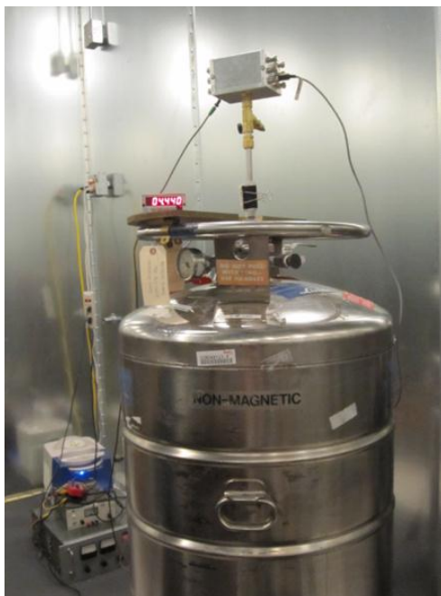
Figure 3.6 Picture of low temperature measurement system in the lab.
