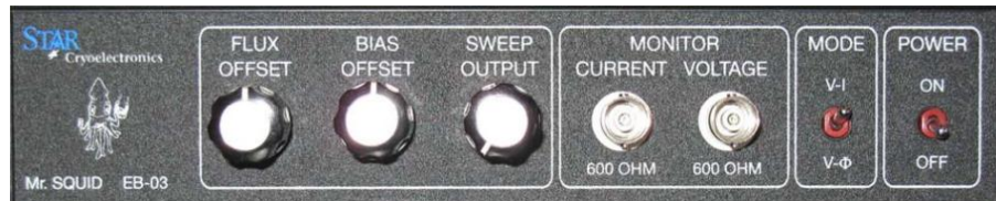
Figure 3.4 Front panel of Mr. Squid box
