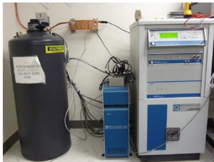
Figure 3.5 Picture of PPMS system in the lab
