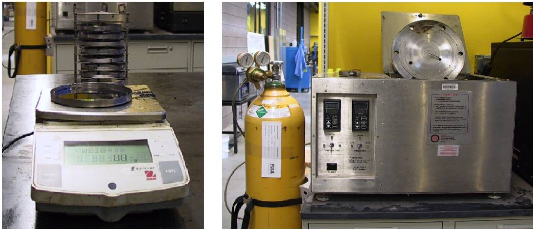
FIGURE 41 PAV equipment and specimen preparation.
