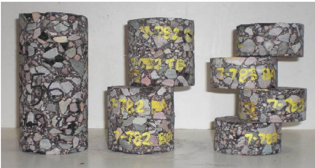
FIGURE 105 Steps of specimen cutting for different air void calculations
