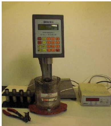
FIGURE 47 Brookfield test apparatus and specimen preparation.
