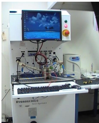
Figure 19. Greenlight Test Station (G50 Fuel Cell System, Hydrogenics, Vancouver, Canada)
