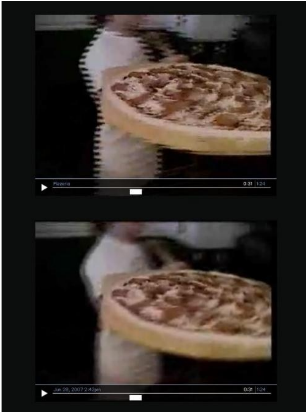
Figure 1-3: Deinterlaced VS Progressive videos streamed on a Facebook Video Stream player. The video on top is an interlaced video, deinterlaced using LA, while the one on the bottom is a progressive video.
