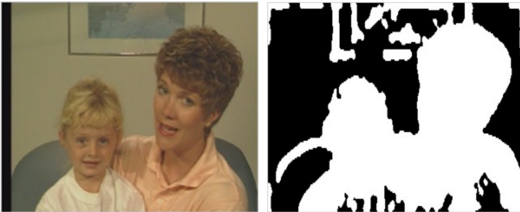
Figure 5-1: Mother video and the detected saliency, post thresholding.
