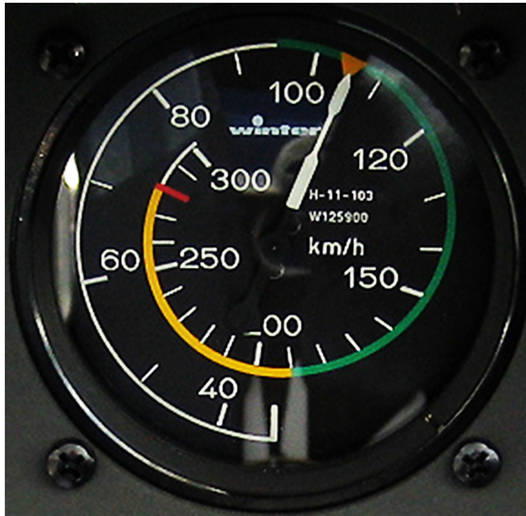
Figure 17: Non-linear airspeed indicator, installed in a high performance sailplane
