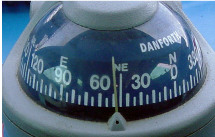
Figure 20: Wet compass, demonstrating non-linear mapping onto the retinal plane of a constantly spaced scale on a curved solid object
