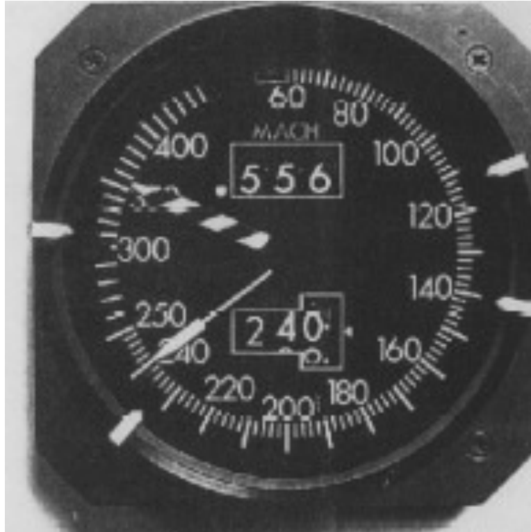
Figure 18: Boeing 757/767 airspeed indicator, reproduced from Hutchins, 2000
