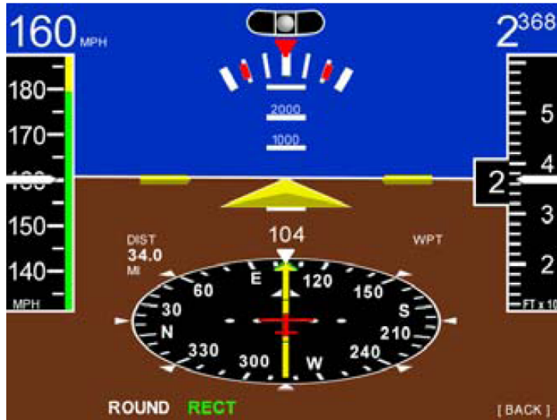
Figure 22: EFIS showing non-circular compass rose, reproduced from TruTrack Flight Systems, 2009
