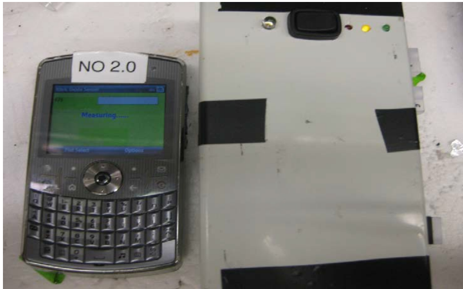
Figure 26. Whistle implemented Asthma Device with cellphone measuring the flow rate & frequency out of Range
