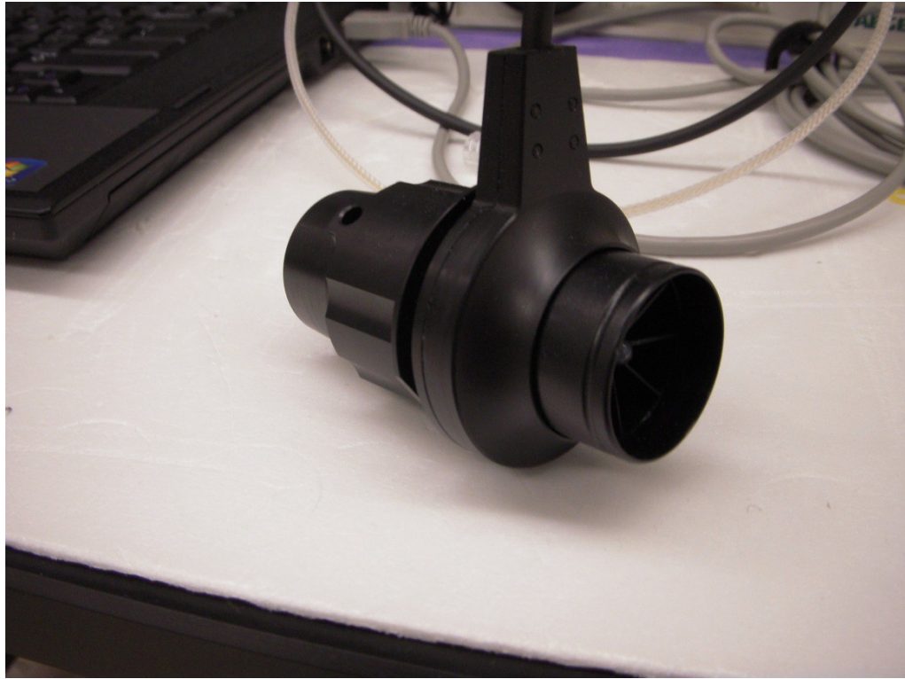
Figure 3: Turbine flow meter employed in Oxycom (Center for Biosensors and Bioelectronics ASU)
