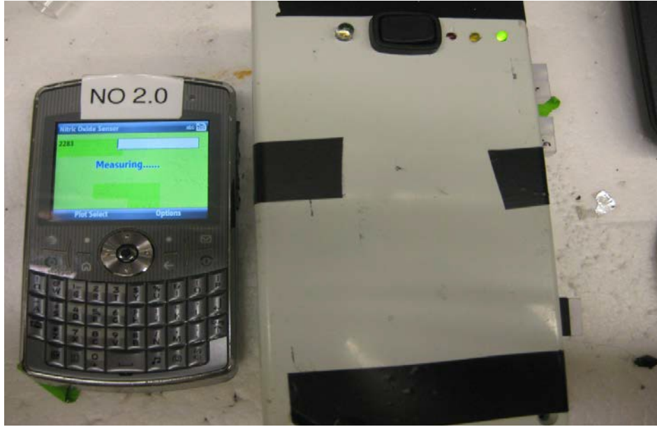
Figure 25. Whistle implemented Asthma Device with cellphone measuring the flow rate & frequency in Range
