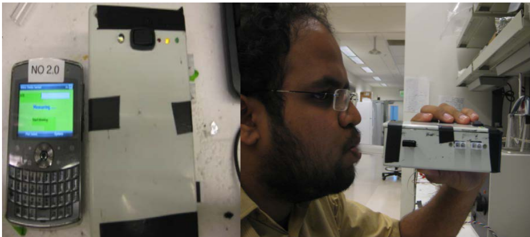
Figure 24. Whistle implemented Asthma Device with cellphone measuring the flow rate
