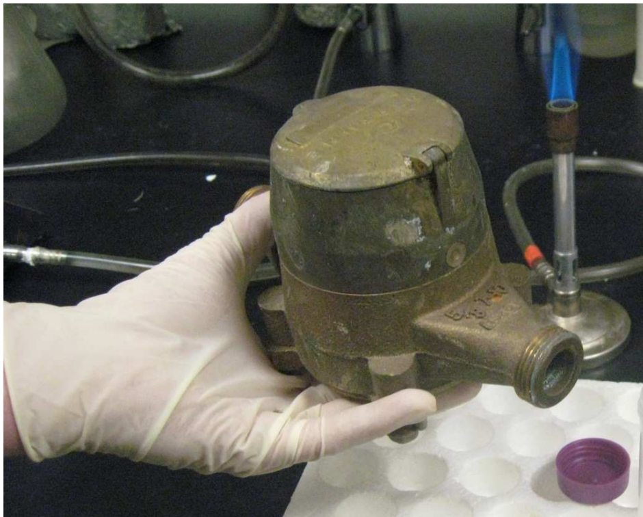
Figure 9- Sample domestic water meter collected from large water distribution system in central Arizona
