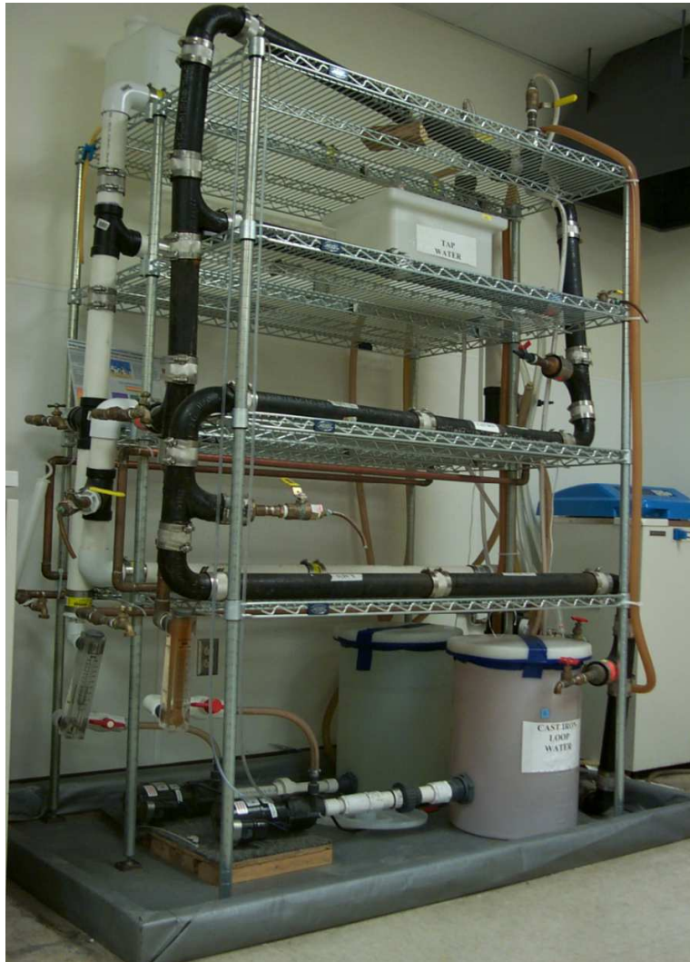
Figure 8-Pilot scale PVC water distribution system (back). Also shown is a cast iron pilot scale water distribution system (front)
