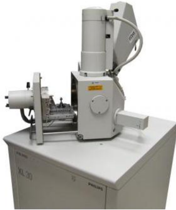
Figure 2.6 Philips XL 30 scanning electron microscopy used at ASU (Courtesy: CSSS, ASU)
