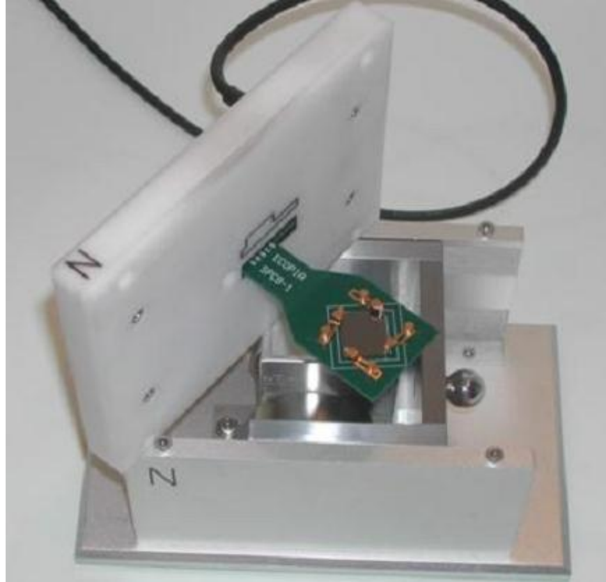
Fig. 2.9 Ecopia HMS-3000 Hall Effect Measurement System used at ASU (Courtesy: ASU)
