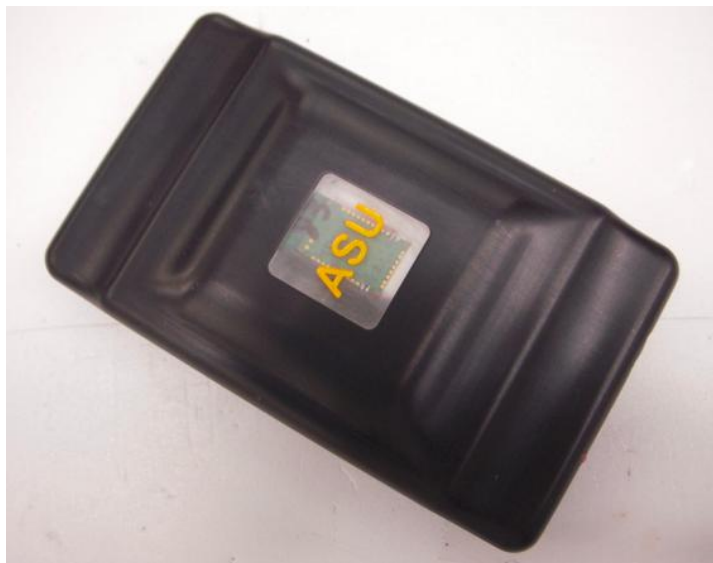
Fig.7. The wireless VOC sensor developed by ASU
