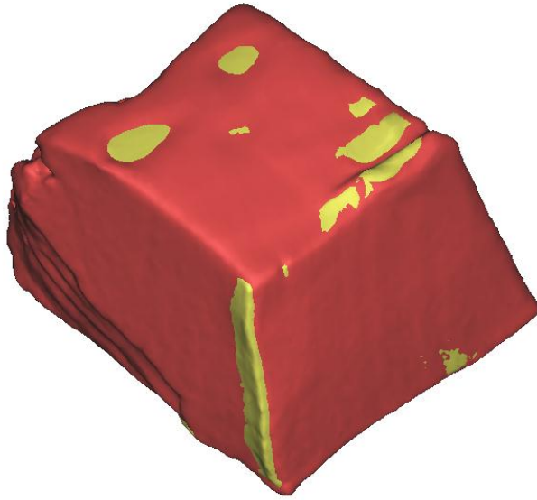
Figure 22: 3D model of solder sample before (yellow) and after indentation (red). The circular yellow areas on the top surface correspond with the indentation sites. While the phase spacing is rather large according to the 2D imagery, there is very low contrast between the phases in the lab scale tomography data. Nonetheless, comparison of the same 2D cross section in the before and after deformation data shown in Figure 23.
