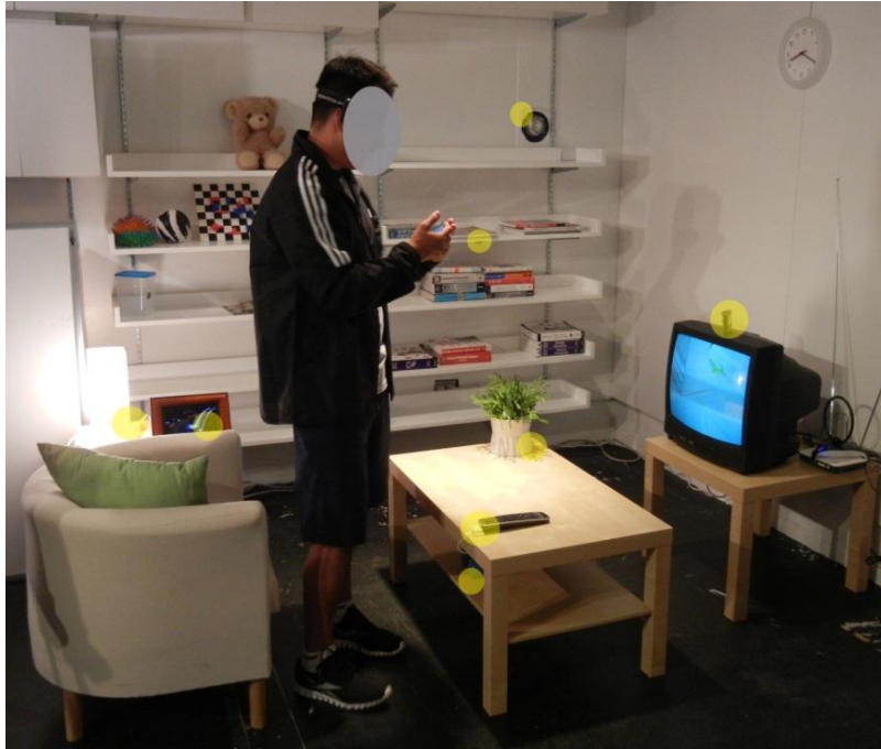
Figure 23. Living room setting and placement of sensors (yellow circles)
