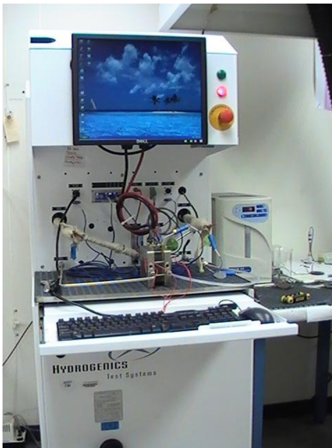
Figure 11 Greenlight test station and single test fuel cell
