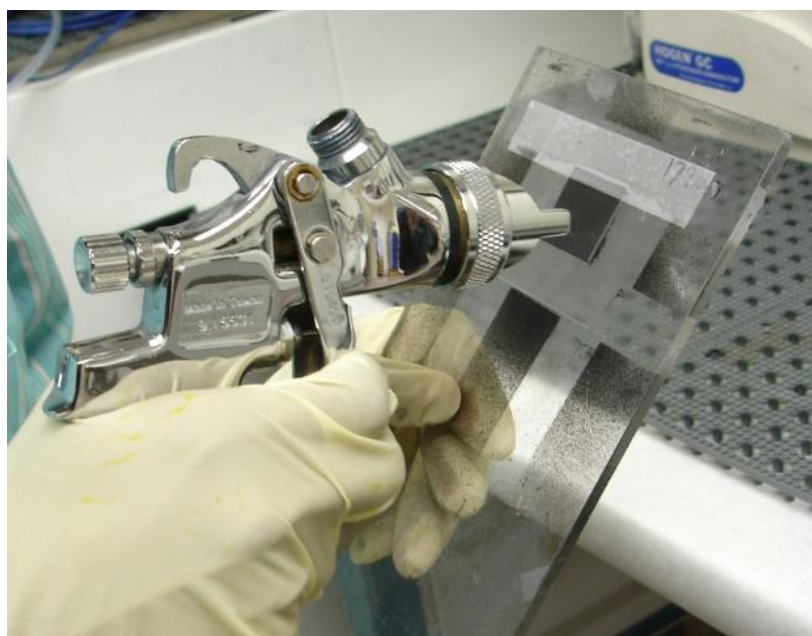
Figure 10 Microspray electrode fabrication method
