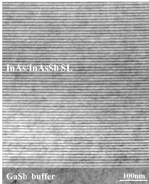
Fig. 5.3. Cross-sectional electron micrograph of Sample A demonstrating the excellent crystallinity of the In InAs/InAs 0.78 Sb 0.22 SL.
