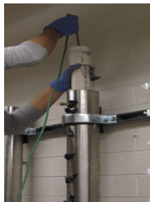
Figure 2.5. Column packing (compressing down the soil)
