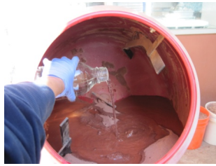
Figure 2.4. Moisturizing and mixing the soil
