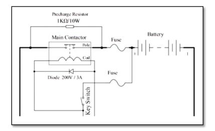
Figure 11. Power solenoid wiring diagram [10].
