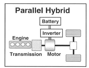
Figure 2. Typical parallel hybrid configuration [3].
