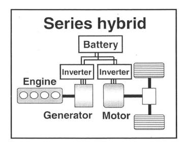
Figure 1. Typical series hybrid configuration [3].
