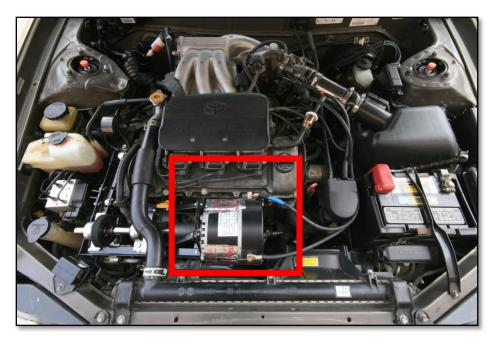
Figure 7. Mars ME0909 PM DC motor mounted above front exhaust manifold.
