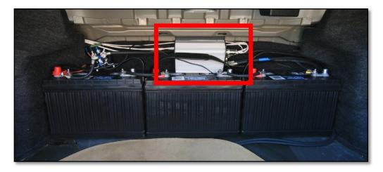
Figure 9. Kelly Controls KDZ48401 PM DC motor controller with regen.
