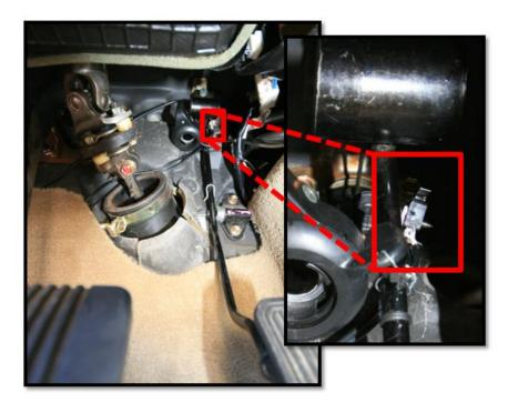
Figure 13. Regen/brake switch mounted behind accelerator pedal arm. 3.3.4 Wires & Power Cable
