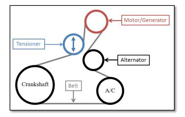
Figure 16. Serpentine belt routing diagram.
