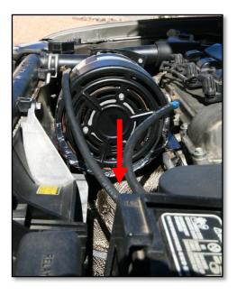
Figure 8. DEI© Titanium Exhaust Wrap.
