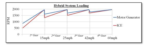
Figure 19. Hybrid system loading under normal acceleration.
