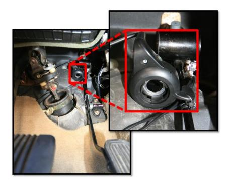
Figure 12. Thumb throttle potentiometer mounted to accelerator pedal.
