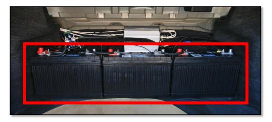
Figure 10. The 36 V EverStart® MAXX battery bank (trunk carpet removed).
