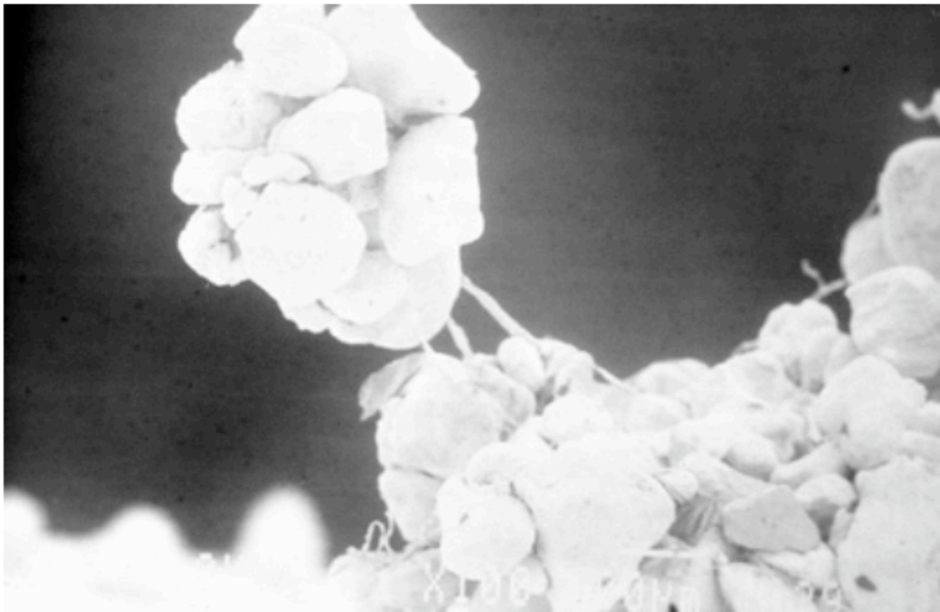
Figure 1-3. Scanning electron micrograph (x100) of a cyanobacterial sheath binding soil particles together (photo courtesy of soilcrust.org). This image highlights the role that cyanobacteria play in soil stabilization, and also displays the intimate association between crust microbes and the soil solid-phase.
