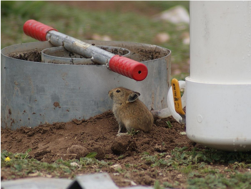
Figure 7. Double ring infiltrometer with a plateau pika in the foreground.
