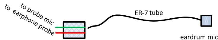
Figure 30. The diagram to calibrate the eardrum microphone with respect to the probe microphone.
