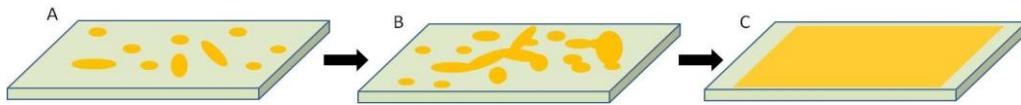
Figure 3.4. Illustration of metal morphology in different stages: In A stage, there are small islands only. In B stage, islands start to connect with each other and form larger conducting paths. In C stage, the surface is an uniform metal layer.
