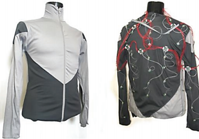
Figure 46. Movie enhancing tactile jacket with 62 vibrotactile actuators distributed across the torso and arms. Reprinted from “A body-conforming tactile jacket to enrich movie viewing,” by Lemmens, P., Crompvoets, F., Brokken, D., van den Eerenbeemd, J., & de Vries, G. J., 2009, In Proceedings of the Third Joint EuroHaptics conference and Symposium on Haptic Interfaces for Virtual Environment and Teleoperator Systems, p. 7. Copyright © 2009 by IEEE. Reprinted with permission.
