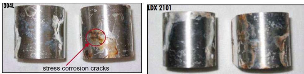
Figure 2.3: Corrosion Test Performed Using ASTM C692 after 672 Hours at 212 0 Fahrenheit
