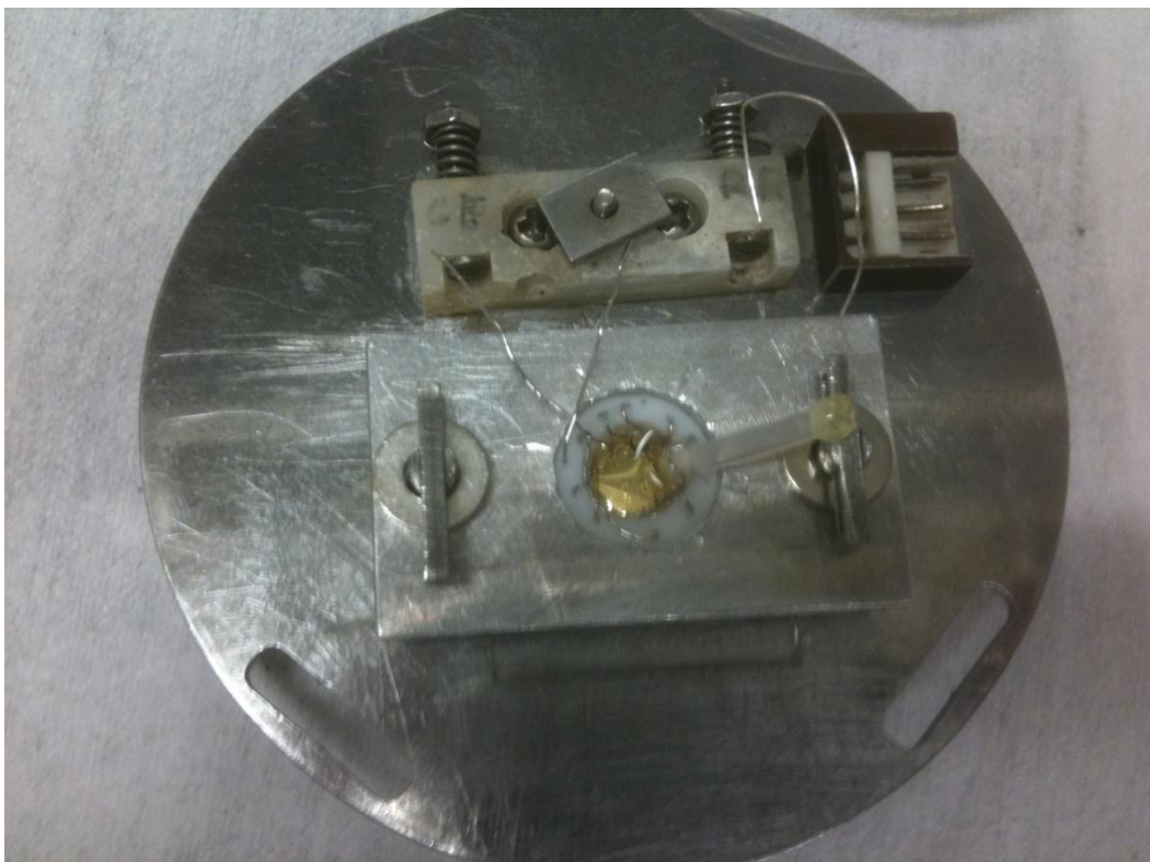
FIGURE 17. Photo of the EC-STM cell employed for these experiments. Counter electrode is woven into the Teflon ® cell and with an electrical connection on the left. A Ag/AgCl reference electrode is on the right and the working electrode is the Au (III) substrate in the center.
