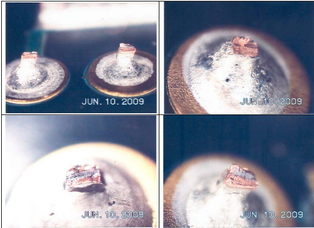
Figure 4.20 DEU-II I/O CCA resistor lead fatigue as seen from the SAC305 solder joint (4 photos)
