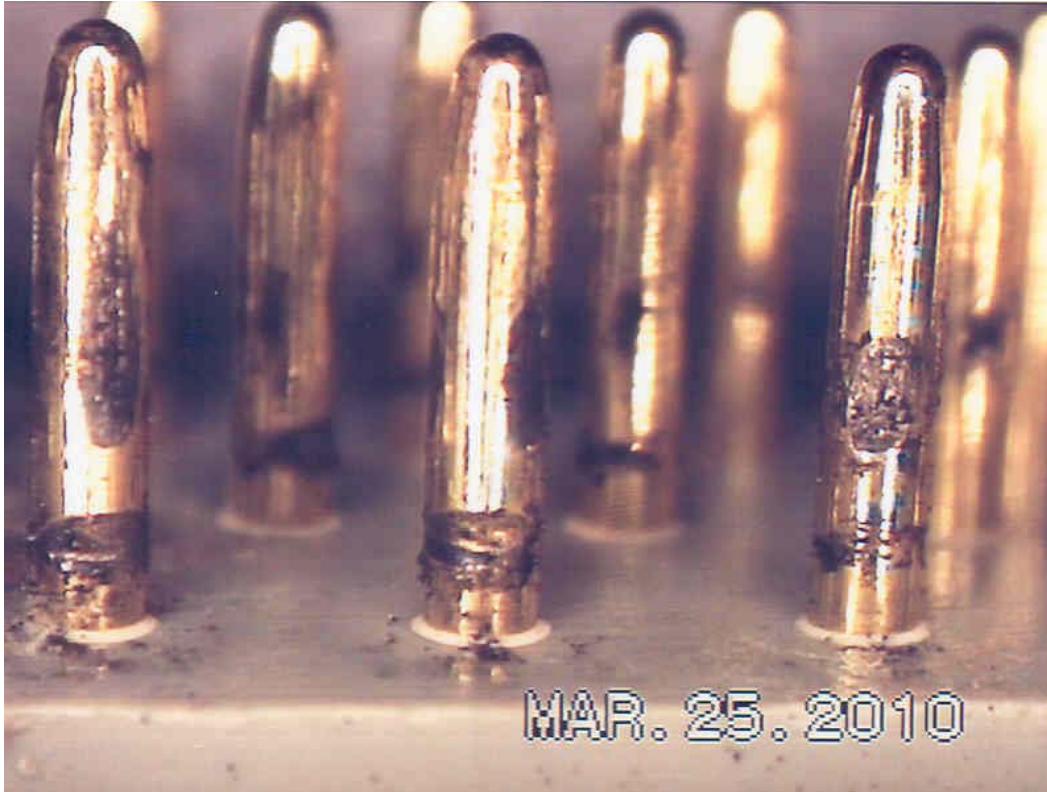
Figure 4.22 SAC305 DEU-II LRU with a Sn-Pb solder power supply showing connector fretting
