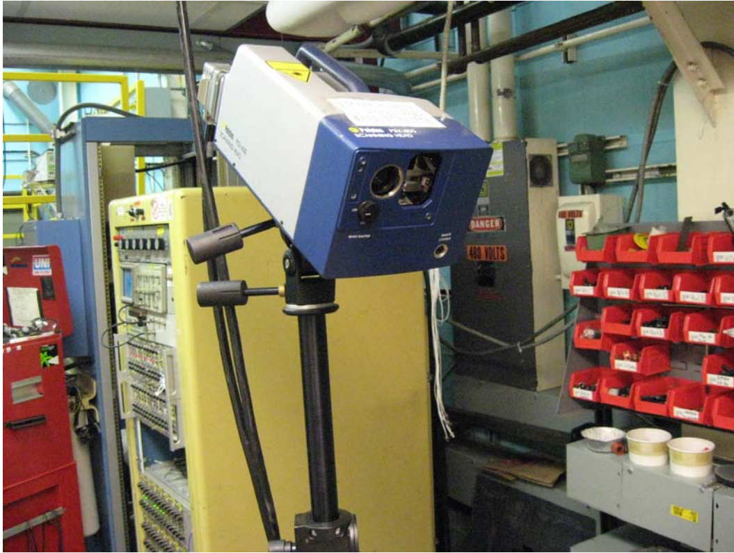
Figure 3.26 Laser Vibrometer system pointing at the test vehicle
