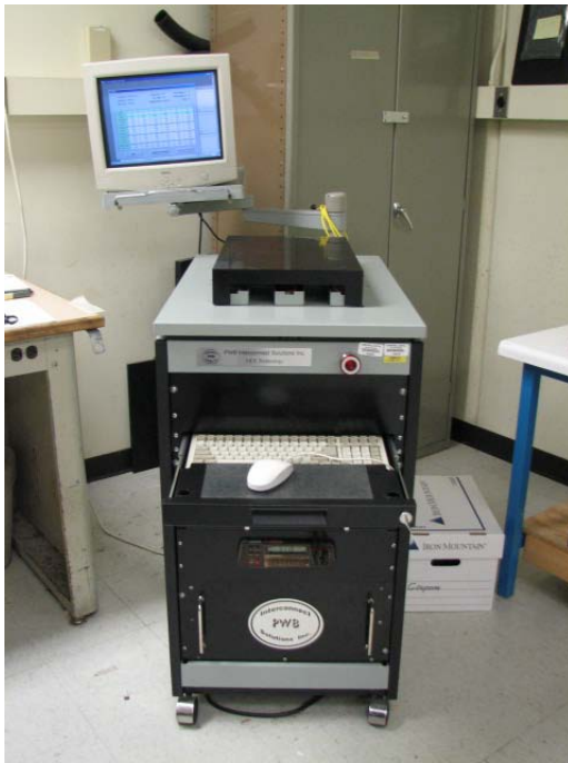
Figure 2.1 IST machine capable of performing both preconditioning and accelerated testing of six coupons at a time.
