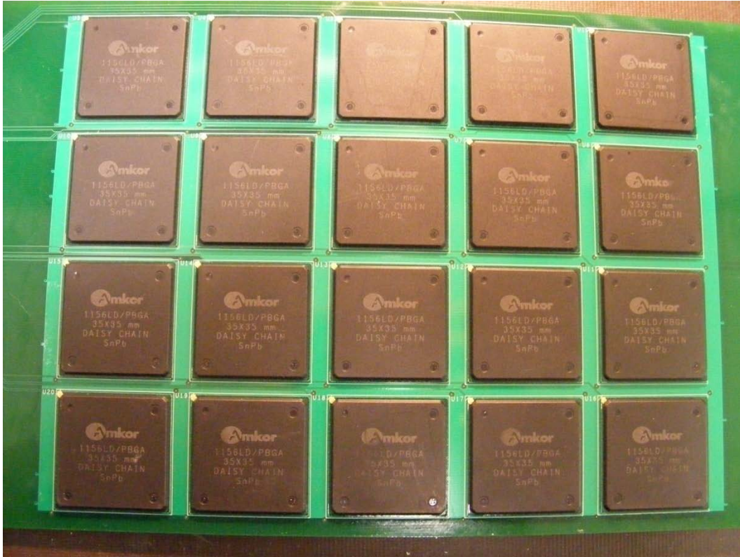
Figure 3.27 Test vehicle with 20 daisy chained 1156 BGAs 35mm x 35mm; location 1 is at the upper right hand corner and locations 2-5 proceed to the left in the upper row; locations 6-10 are in the second row; locations 11-15 are in the third row; and locations 16-20 are in the bottom row, where location 20 is on the bottom left hand corner. The numbers can be made out in the picture with designations going from U1-U20
