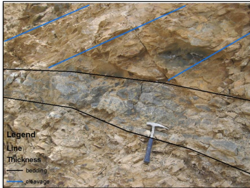
Figure 21. Image from the Main Pit of S2 cleavage cutting across bedding (S1 is not present at this location). Bedding is shown with black lines, while cleavage is shown with blue lines.
