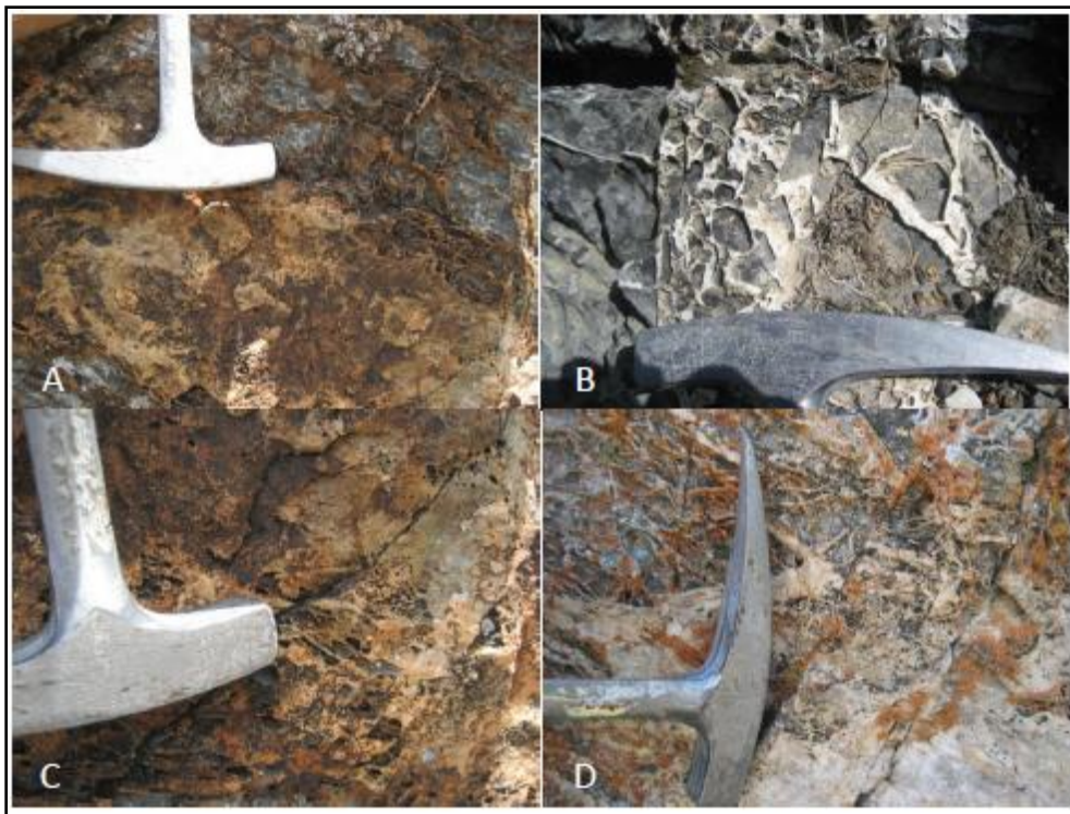
Figure 30. Various observed intensities of quartz-vein flooding from the Lamb Dolomite south of the Mined Strip. Image A shows quartz stockwork in upper right grading into quartz flooding. Image B shows quartz veins as matrix to a crackle breccia. Image C shows fragments of stockwork quartz in a zone flooded with quartz. Image D shows the sharp gradation from quartz stockwork to quartz flooding.
