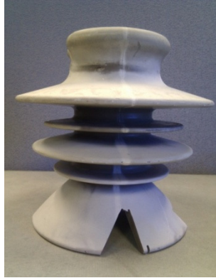
Figure 16. Schematic of standard 10 kV pin type insulator
