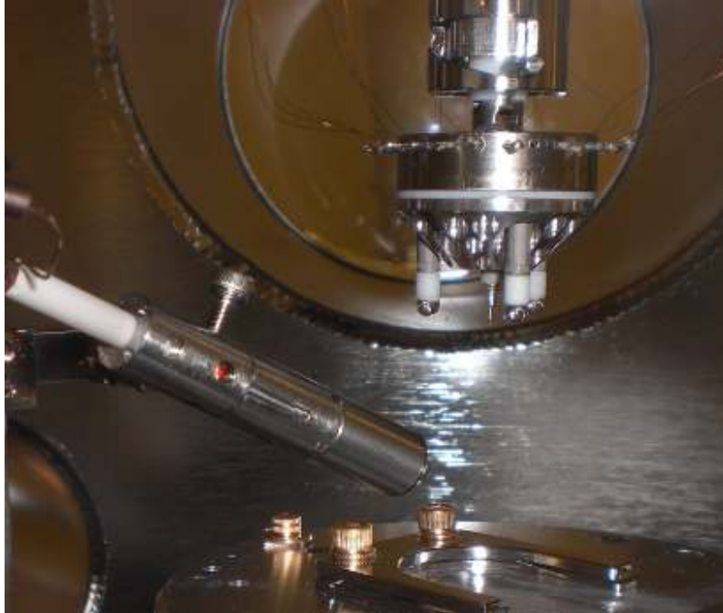
Fig. 5.4 A cylinder type enclosure of the deposition source is aiming to the center of the STM stage. The deposition source unit is inserted into the back side of the enclosure. The STM sample holder is not shown in the picture.
