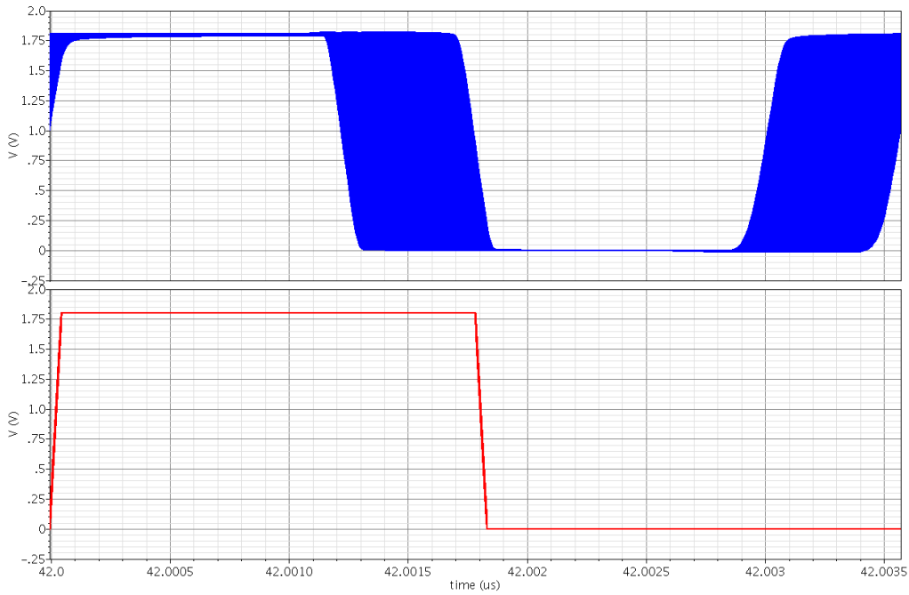
Figure 81. Persistence plot without DLL with 20 mVpp, 1 MHz supply noise (BSIM 3.3 DCO, Kp=4, Ki=1).
