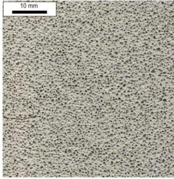
Figure 29: Cross Section of a 2 × 2 in. AFRC sample (Bonakdar and Mobasher 2010)
