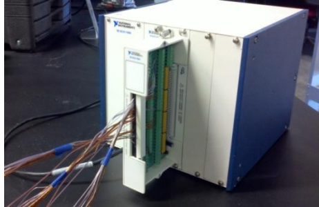
Figure 26: National Instruments Data Acquisition System with Thermocouples
