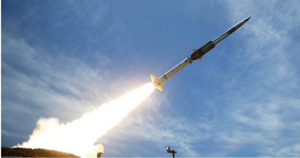
Figure 6: Orbital Sciences' GQM-163A Coyote Supersonic Sea Skimming Target using a residual Mk70 solid rocket motor booster. 21
