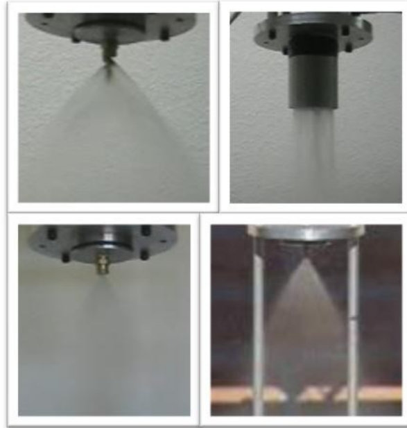
Figure 42: Clockwise from upper left: spiral flow valve, sidewall impingement on pre-catalyst bed chamber, cone spray with water, cone spray with HAN.
