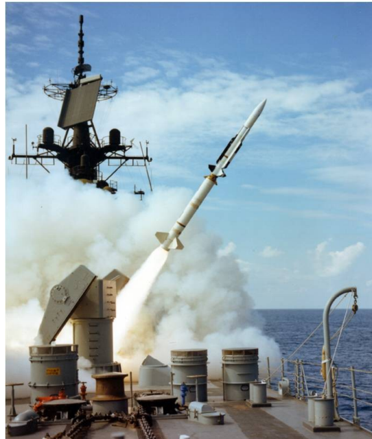
Figure 17: A Standard Missile 2 (SM-2) composed of a Mk70 booster and a Mk30 sustainer is launched from a U.S. Navy Aegis Combat System Destroyer. 41
