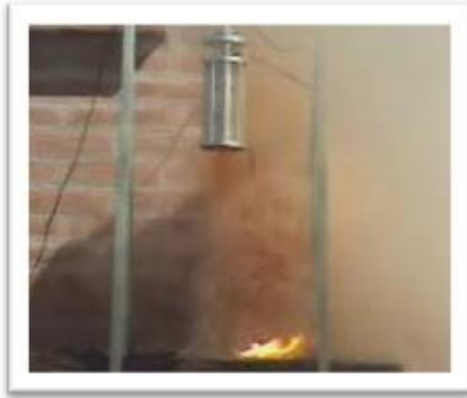
Figure 47: Hang-fire of motor during initial ignition trials.
