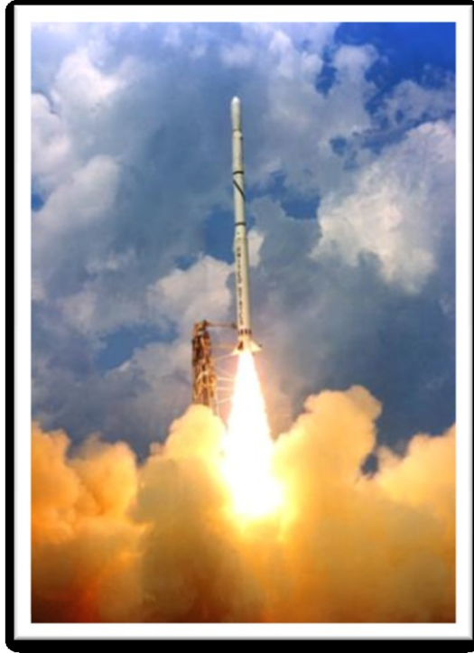
Figure 5: Scout vehicle composed of four solid rocket motors.
