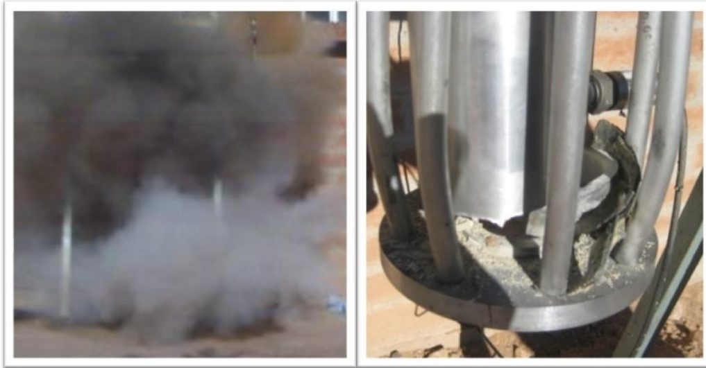
Figure 50: Left: Over-pressurization of HAN Solo v.1 following sustained thrust trial. Right: aftermath of over-pressurization.
