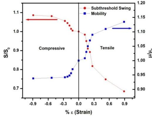
Fig. 4.10. Relative  $S$  and  $\mu$  as function of applied strain ( $\epsilon$ ).  $V_{GS}$  varying from - 20 to 20V.
