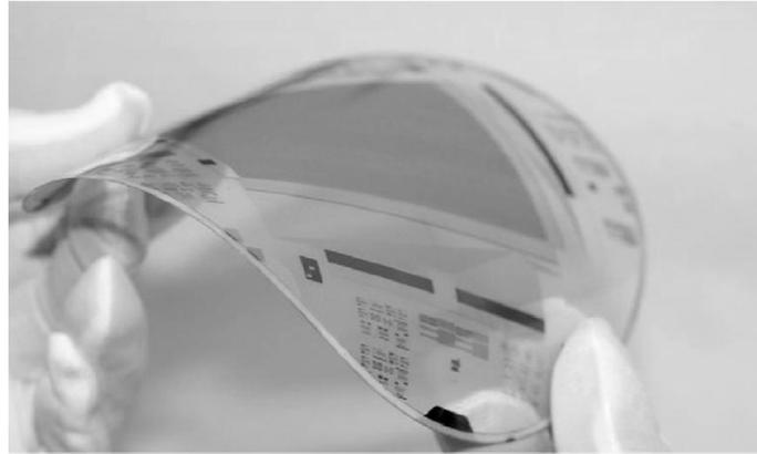
Fig. 2.2 QVGA electrophoretic display backplane on plastic.
