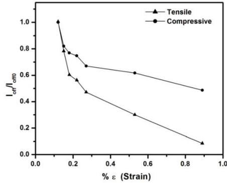
Fig. 4.11. Relative  $I_{off}$  due to tensile and compressive stress vs % strain ( $\epsilon$ ).  $V_{GS}$  varying from - 20 to 20 V at  $V_{DS} = 10V$ .
