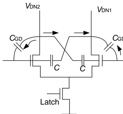
Fig. 7.2. Self neutralization technique using extra  $C$ .
