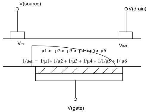
Fig. 4.5. Schematic showing effective mobility and  $V_{th}$  across channel in post stressed forward and reverse currents.
