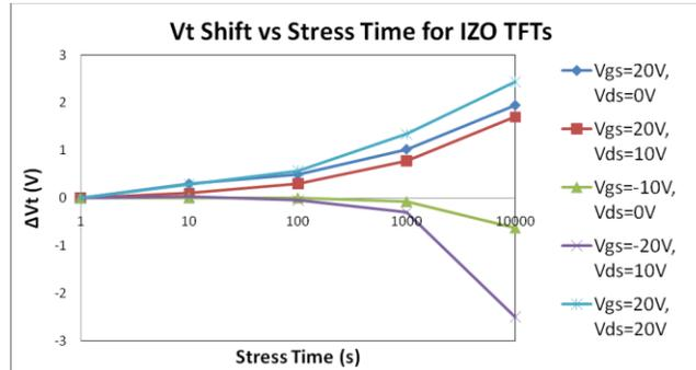
Fig. 4.1 Change in  $V_{th}$  after 10,000 seconds of DC stress for ZIO TFTs.
