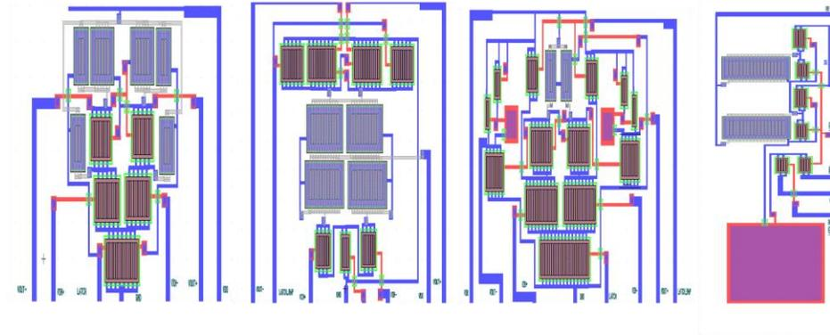
Fig. 8.2. Layout of different comparators for flash ADC in CMOS TFTs.
