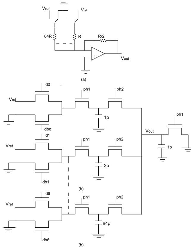
Fig. 6.2. Circuit Schematic of 7 bit switched cap DAC.
