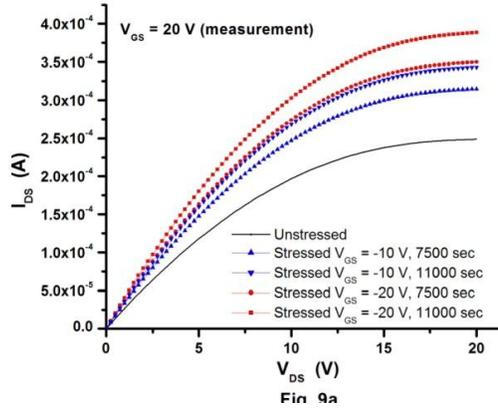
Fig. 4.9a.  $I_{DS}$ - $V_{DS}$  characteristics. Negative bias stress.
