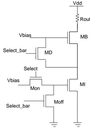
Fig.6.8. Cascode current source in current steering DAC.
