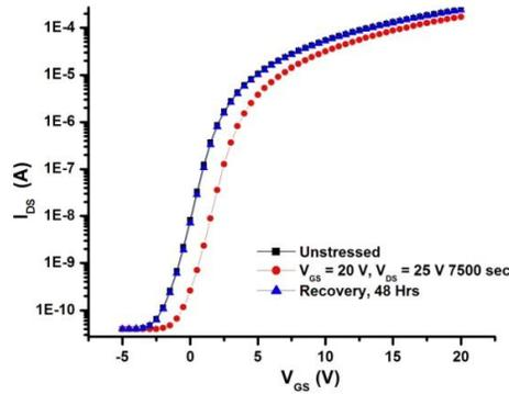
Fig. 4.8. Transfer characteristics recovery for  $V_{GS} = 20$  V and  $V_{DS} = 25$  V stress.
