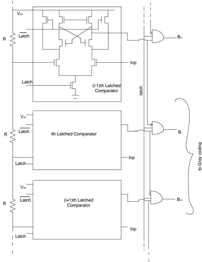
Fig. 7.3. Block diagram of the 5 bit ADC.
