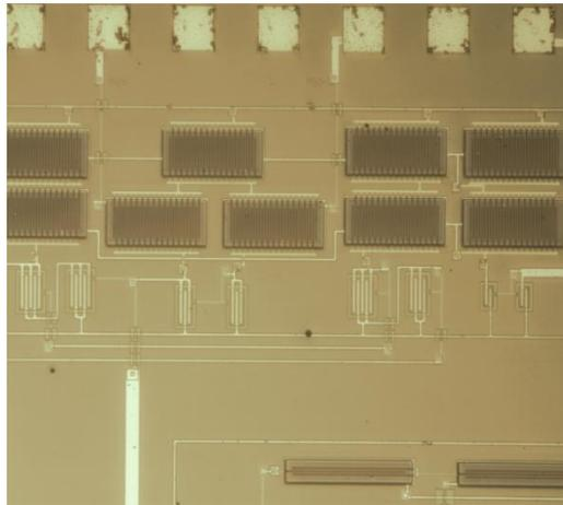
Fig. 5.1 p-channel input 2 stage op-amp fabricated with amorphous silicon and pentacene TFTs.
