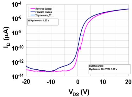
Fig. 3.2. Measured transfer characteristics of a-Si:H TFTs.
