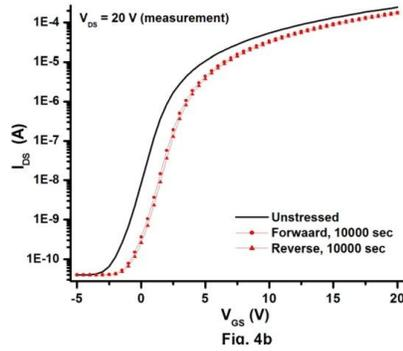
Fig. 4.4b.  $I_{DS}$  vs  $V_{GS}$  plot. Stressed in saturation mode.
