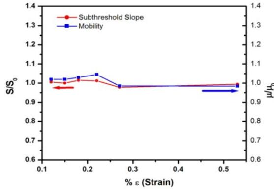
Fig. 4.14. Relative  $S$  and  $\mu$  as function of the applied  $\perp$  strain ( $\epsilon$ ).  $V_{GS}$  from - 20 to 20 V.
