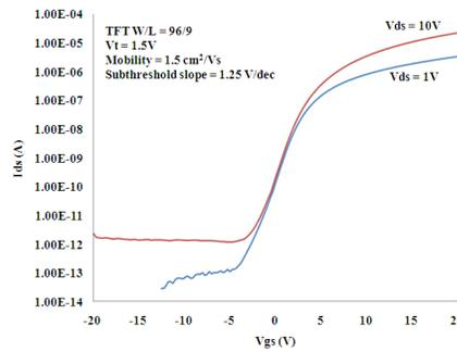
Fig. 3.8. Measured transfer characteristics of a-ZIO TFTs.
