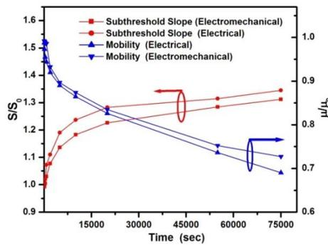
Fig. 4.13. Electrical and tensile electro-mechanical stress (dia = 5.08 cm,  $\epsilon = 0.27$  %).
