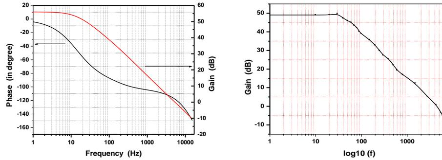
Fig. 5.3a) Simulated gain and phase vs frequency response; b) Measured gain response of fabricated op-amp.
