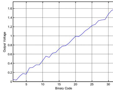
Fig. 6.12. Linearity curve obtained from DAC.
