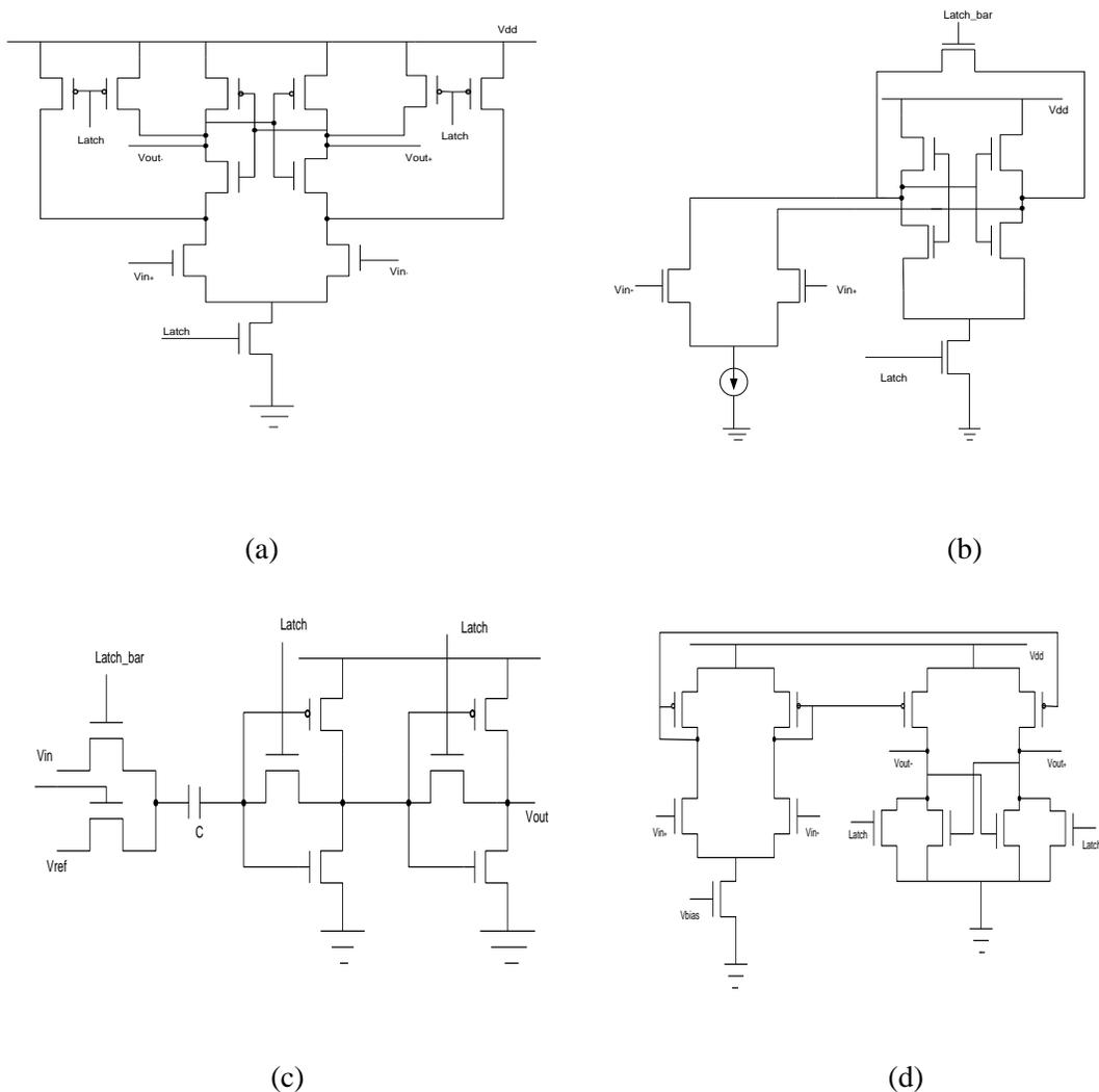
Figure 7.1 Comparators for flash ADC: (a) Class AB, (b) Dynamic, (c) Auto-zeroed and (d) Class A.
