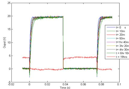
Fig. 2.10 Degradation of inverter characteristics with time after [13].
