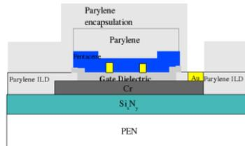
Fig. 3.4. Cross section of pentacene TFT structure with different layers.
