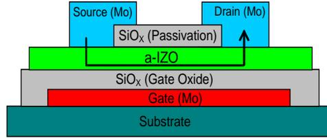
Fig. 3.7. Cross section of a-ZIOTFT structure with different layers.
