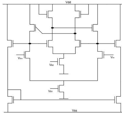
Fig. 2.12 Schematic of an all nMOS op-amp with gain boosting after [19].
