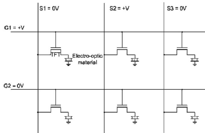
Fig. 2.3 Active Matrix on a-Si:H backplane.
