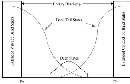
Fig. 3.3. Band tail and deep states within a-Si:H bandgap.
