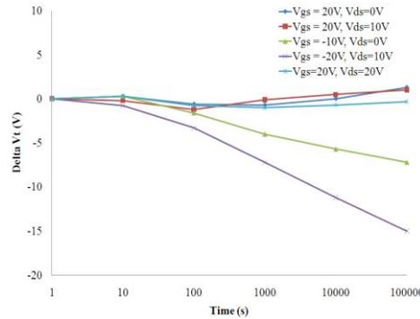
Fig. 5.6 Change in  $V_{th}$  with constant DC stress of ZIO [62].
