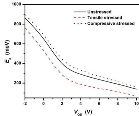
Fig. 4.12. Activation energy vs gate bias (bending diameter = 5.08 cm,  $\epsilon = 0.27\%$ ).
