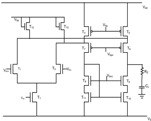
Fig. 5.4 Folded cascode nMOS input OTA.
