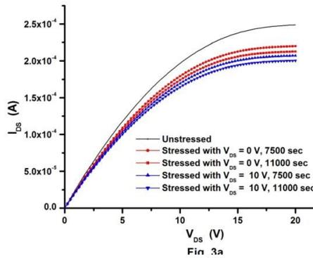
Fig. 4.3a. Stressed in linear mode.  $V_{GS} = 20$  V and  $V_{DS} = 10$  V. Forward and reverse mode currents coincide.
