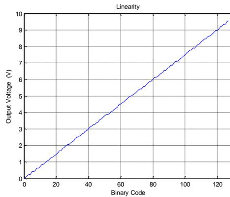
Fig. 6.6 Linearity curve from switched capacitor DAC.
