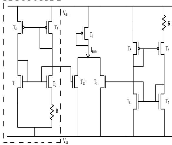
Fig. 5.7 Modified constant  $g_m$  biasing circuit.
