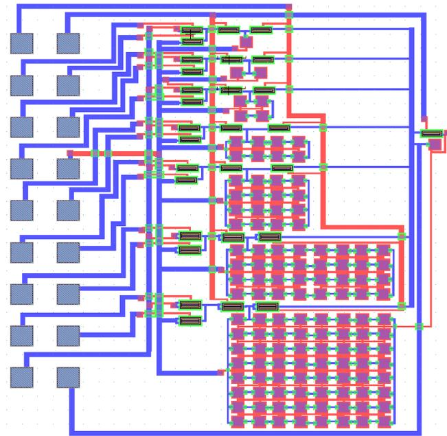
Fig. 6.3 Layout of the DAC.
