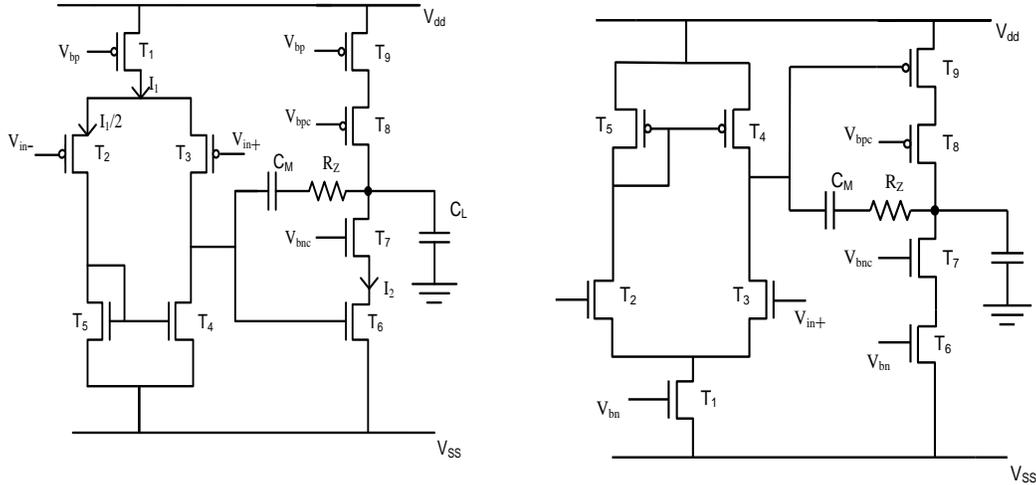
Fig. 5.2a) 2 stage Miller compensated OTA with pMOS 1<sup>st</sup> stage; b) 2 stage Miller compensated OTA with nMOS 1<sup>st</sup> stage.
