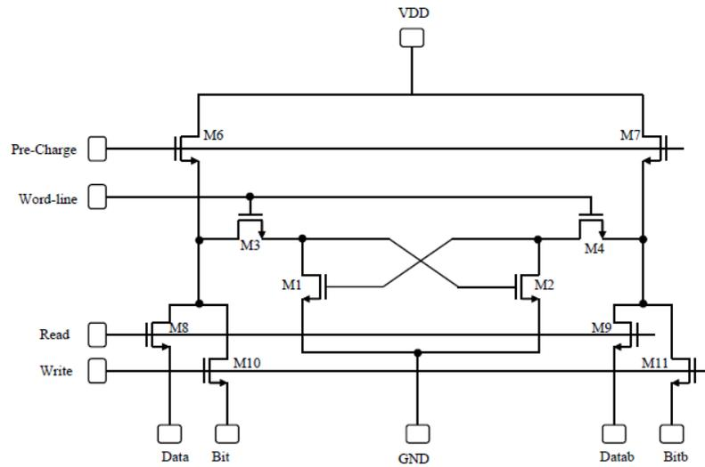
Fig. 2.7. Schematic of all nMOS non-volatile memory after [10].
