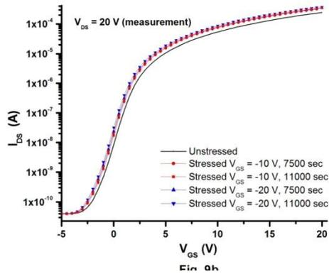
Fig. 4.9b.  $I_{DS}$ - $V_{GS}$  characteristics. Negative gate bias stress. Both forward and reverse mode currents coincide.
