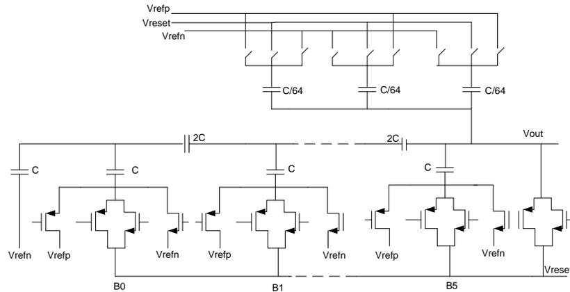
Fig. 2.13 6 bit C-2C DAC after [20].
