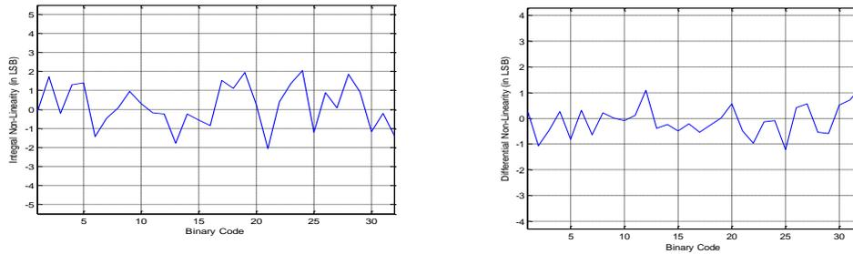
Fig. 6.11 (a) INL and (b) DNL characteristics.
