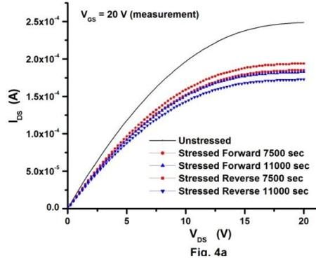
Fig. 4.4a.  $I_{DS}$  vs  $V_{DS}$  plot. Stressed in saturation mode.  $V_{GS}=20$  V and  $V_{DS} = 20$  V.
