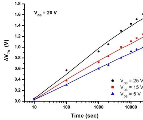
Fig. 4.7. Degradation of  $\Delta V_{th}$  vs time and bias stress. Symbols indicate measured data.
