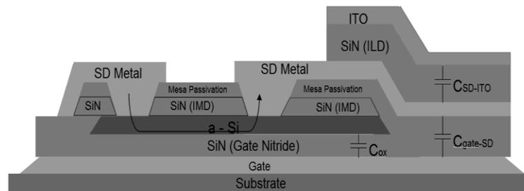
Fig. 3.1. Cross section of a-Si:H TFT structure with different layers.
