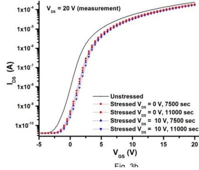
Fig. 4.3b.  $I_{DS}$  vs  $V_{GS}$  plot. Stressed in linear mode showing same current in both modes.
