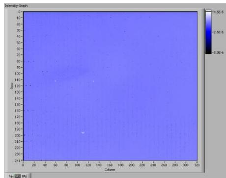
Fig. 6.1 Distribution of  $I_{DS}$  across the wafer from FDC.
