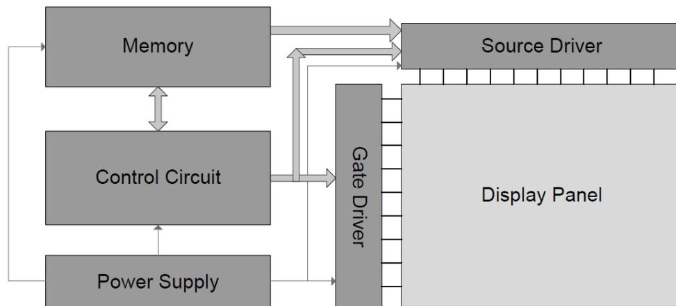
Fig. 2.1 Architecture of a flat panel display.
