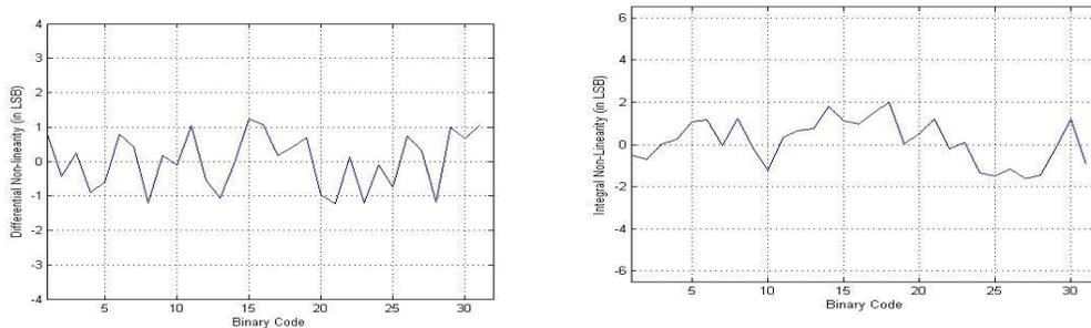
Fig. 7.5 (a) Measured DNL and (b) measured INL from 5 bit ADC.
