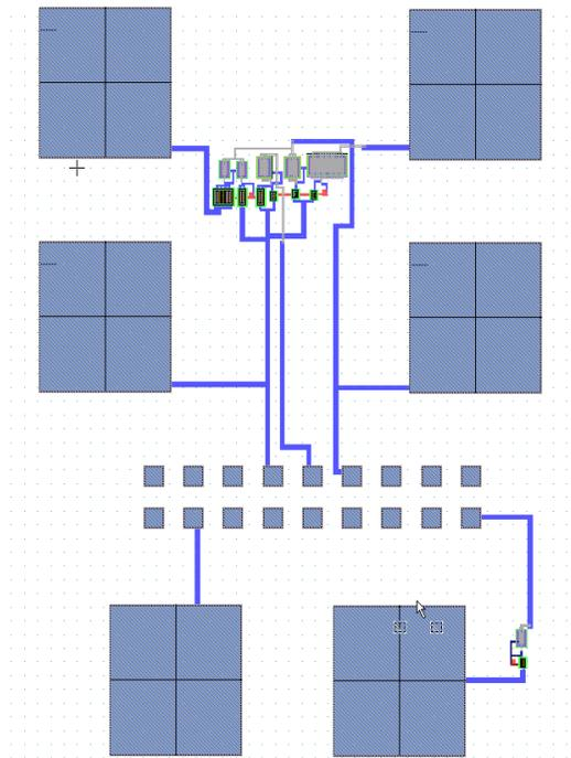
Fig. 8.1. Layout of the novel biasing circuit in CMOS TFT.
