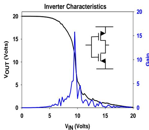
Fig. 2.9 Inverter characteristics and gain on flexible CMOS after [13].
