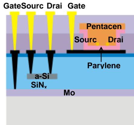
Fig. 3.6. Cross section of a-Si:H/pentacene CMOS TFT with different layers after [13].
