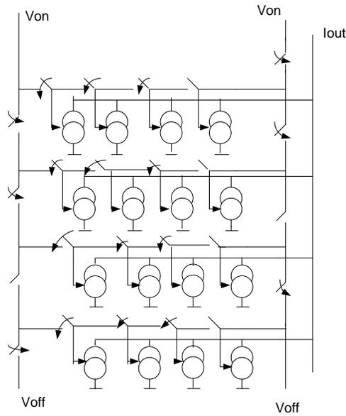
Fig. 6.9. 4 bit array of current steering DAC with 1011 input code.
