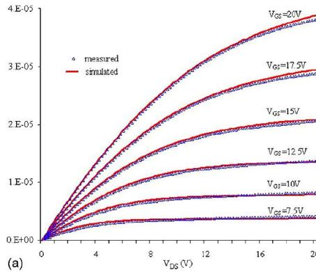
Fig. 2.16. Comparison of measured data with that obtained from the model.
