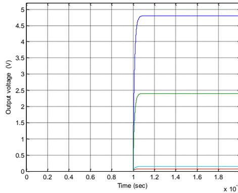
Fig.6.7 Output response with the bits changing from 0 to 1, one at a time with other bits at logic 0.
