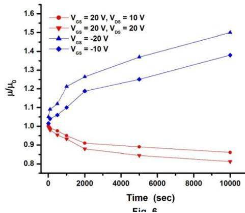
Fig. 4.6. Relative mobility change due to gate & drain bias stress with time ( $\mu_0$  is the virgin mobility).
