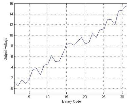
Fig. 7.6 Measured linearity of 5 bit flash ADC.
