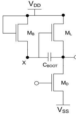
Fig. 2.4 Schematic of bootstrapped inverter.
