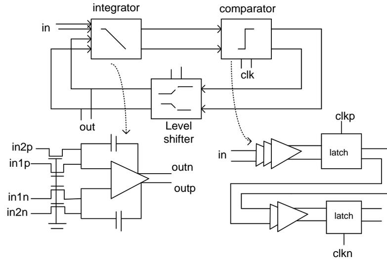
Fig. 2.15. 1<sup>st</sup> order continuous time  $\Sigma\Delta$  ADC in OTFT after [23].
