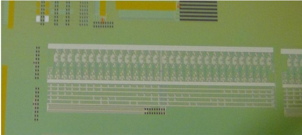
Fig.7.4. Chip micrograph of the full 5 bit ADC with 31 comparators and Gray coding at output.
