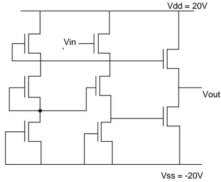
Fig. 2.11 Cascode common source amplifier after [18].
