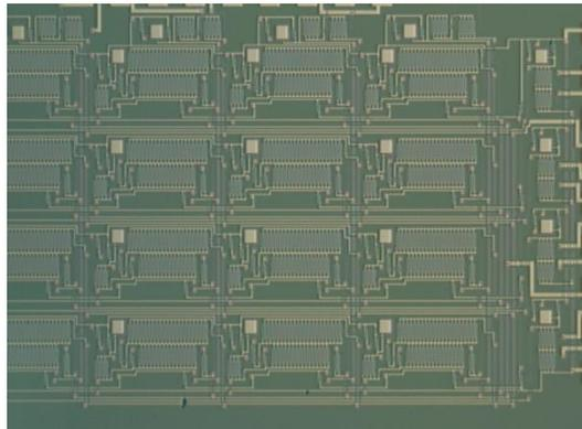
Fig. 6.10. Chip micrograph of 5 bit current steering DAC architecture.
