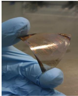
Fig. 2.8 Flexible CMOS logic circuit after [12].
