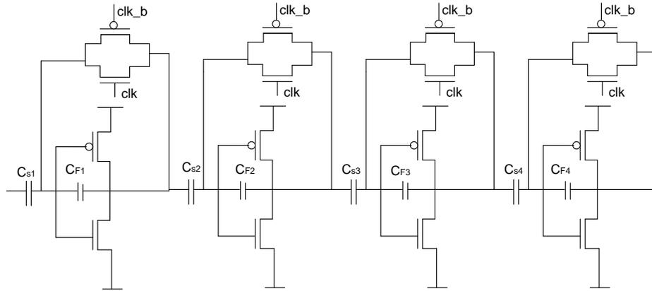
Fig. 2.14 Comparator for 6 bit SAR ADC after [22].
