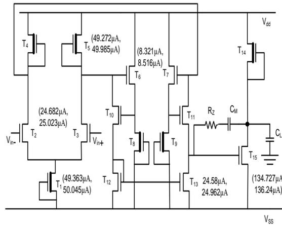
Fig. 5.5 All n-channel enhancement-depletion topology.
