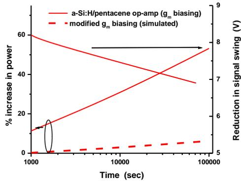
Fig. 5.8. Increase in power and reduction in signal swing using constant  $g_m$  biasing circuit, as the TFTs age with electrical usage. The red dashed line shows reduced degradation for a-Si:H/pentacene using the novel bias circuit.
