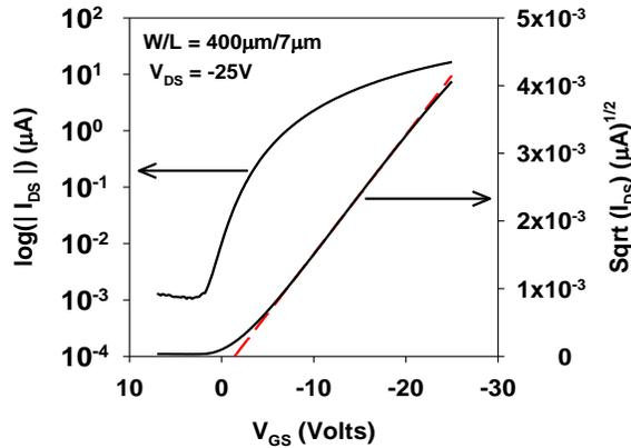
Fig. 3.5. Measured transfer characteristics of pentacene TFTs.
