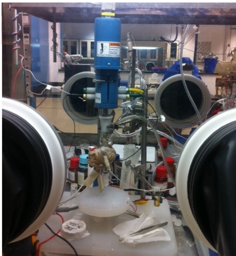
Figure 3.2: Photograph of RRDE cell for super acid titrations. Cell is located in an M-Braun glove box with less than 0.1 ppm atmospheric water.
