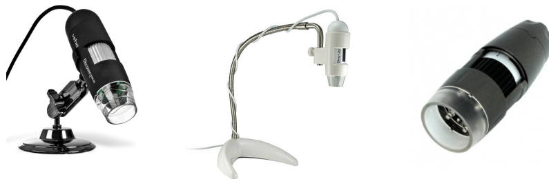
Figure B. 1 Examples of Stands for Inexpensive USB Microscopes Left: USB stand with a heavy base and cradle to hold the microscope. Middle: Flexible metal tubing is creatively used to hold this microscope. Right: This microscope came with no stand at all.
