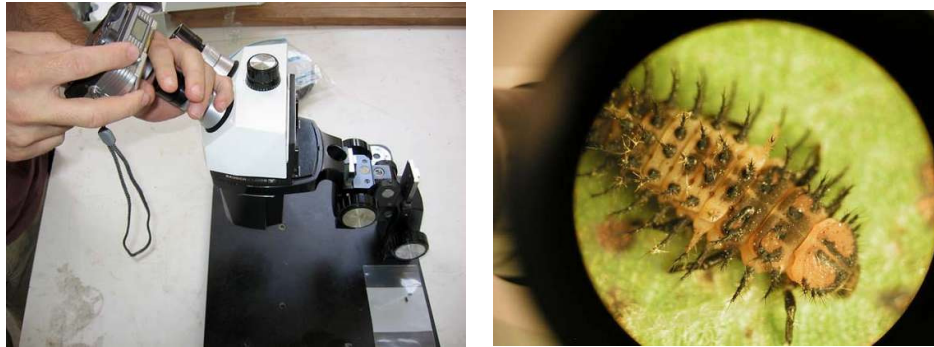
Figure M 4 Holding a Camera to a Microscope Ocular, Resulting Image at Right
