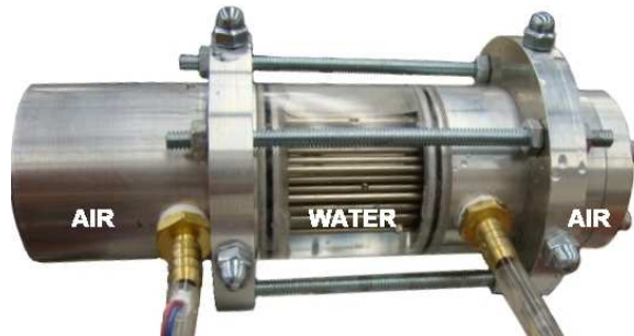
Fig. 2.9. Fabricated heat exchanger with separate air and water chambers
