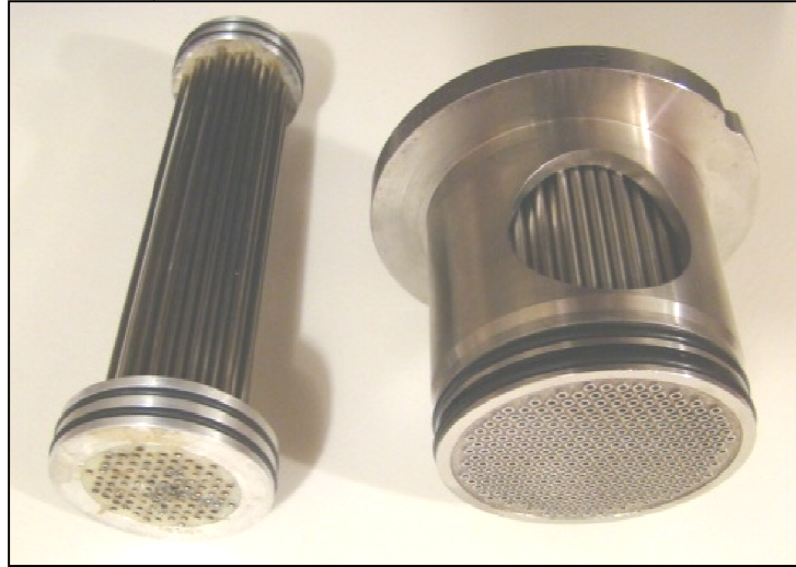
Fig. 2.2. Comparison of the fabricated cooler (left) to an STM 4-120 cooler (right)
