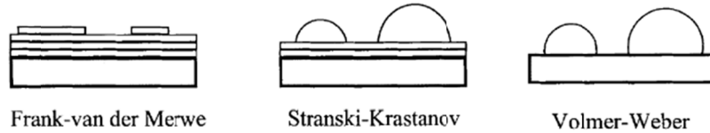
Figure 1. Three basic growth modes in thin films [13]
