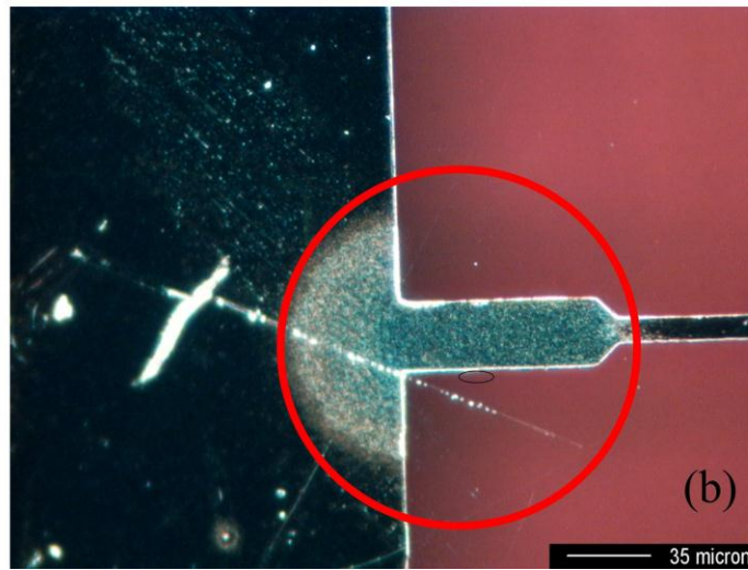
Fig. 19. (a) Time-to-failure as a function 1/V shows a linear relationship. (b) Image using differential interference microscopy shows the site of failure of the interconnect to be at the end where the higher voltage is applied. The site shows a change in thickness in the circled region.
