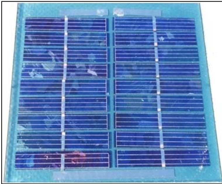
Figure 3.1 Polycrystalline silicon solar cell sensor (rating: 1 W and about 170 mA short-circuit current under standard test conditions)
