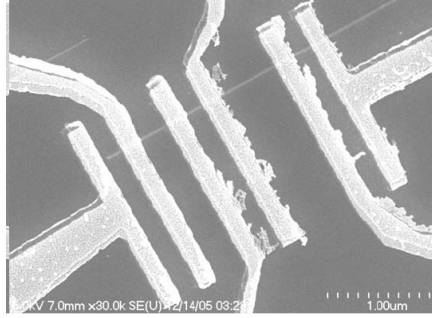
FIG. 4. 2. SEM image of contacts on a NW. The contacts were added ex situ (after growth of the NWs in UHV) by electron beam lithography.
