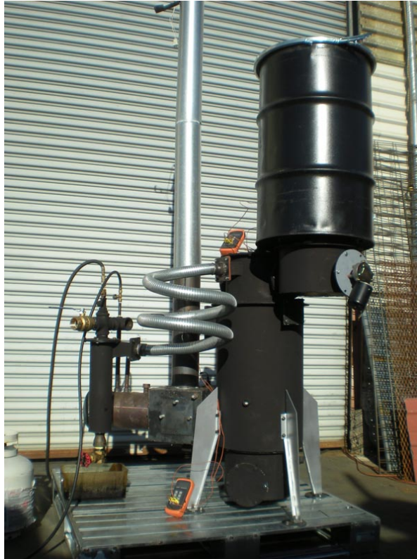
Figure 2. Photo of Biochar Experimenter's Kit continuous pyrolyzer.
