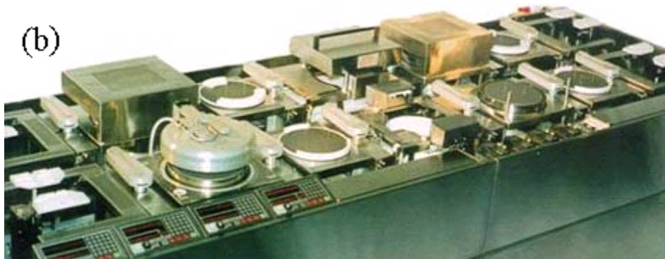
Figure 1.9: Images of (a) automated batch processing wet etch hood and (b) photorealist coater and developer track
