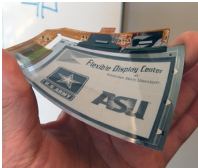
Figure 1.6: Flexible display produced on 125 \mu\text{m} thick stainless steel foil
