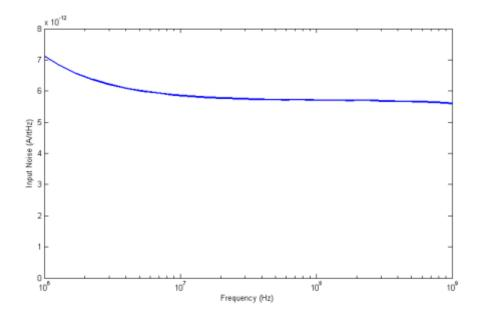
Fig. 29: The spectral density of the OTA noise referred to the input of the TIA.
