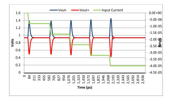
Fig. 31: Transient simulation of complete current showing DC offset cancellation
