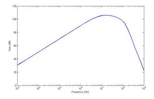
Fig. 30: Gain and bandwidth of complete circuit.
