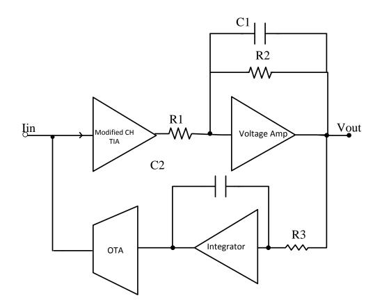
Fig. 16: Block diagram of the presented design.
