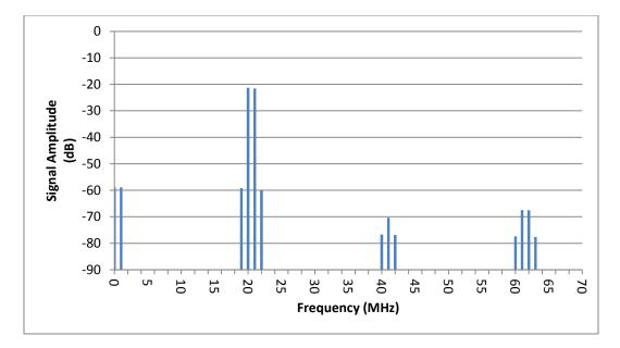
Fig. 24: Third order intermodulated distortion of the TIA.
