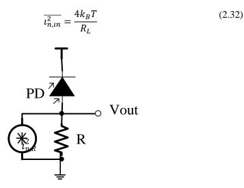
Fig. 4: Photodiode and resistor with noise sources.
