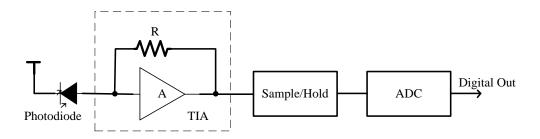
Fig. 1 A block diagram of a general photodiode receiver circuit
