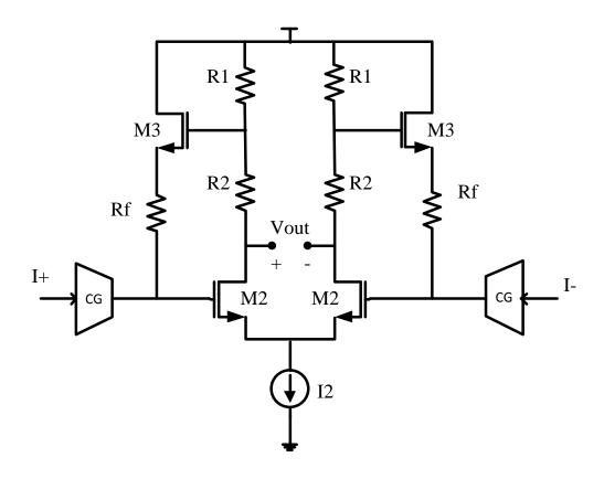
Fig. 14: Schematic of a modified CH TIA.
