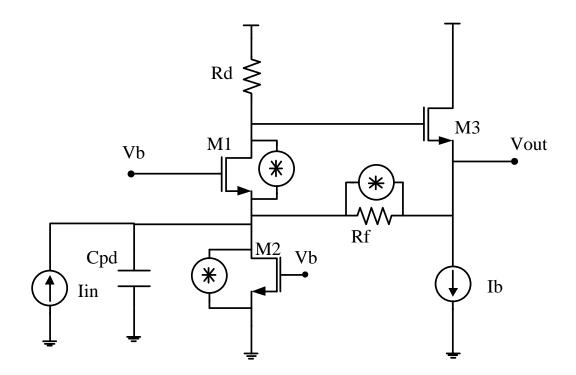
Fig. 7: Common gate amplifier with major noise sources shown.
