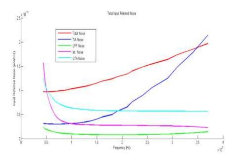
Fig. 32: Superposition of all noise sources compared to total input referred noise.
