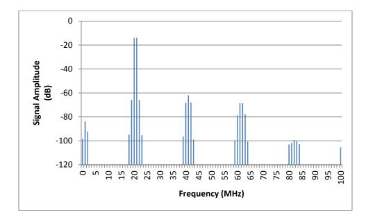
Fig. 33: The intermodulated distortion of the complete circuit.
