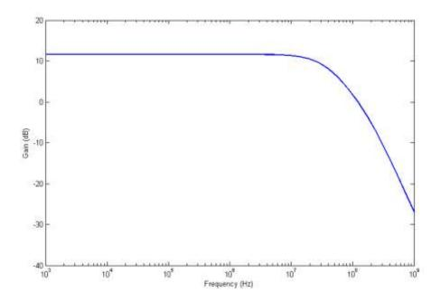
Fig. 25: Gain and bandwidth of the LPF.
