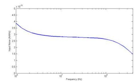
Fig. 28: The spectral density of the integrator noise referred to the TIA input.
