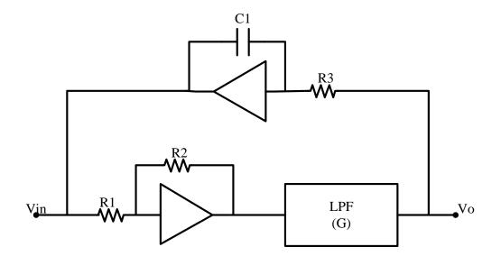
Fig. 15: A block diagram of a voltage amplifier with a servo loop.
