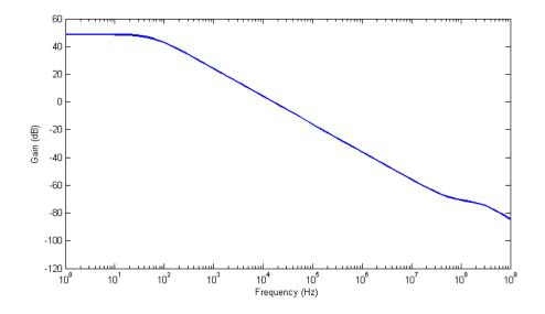
Fig. 27: Gain and bandwidth of the integrator.
