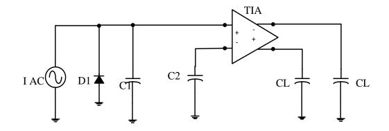
Fig. 21: Test bench for the TIA.
