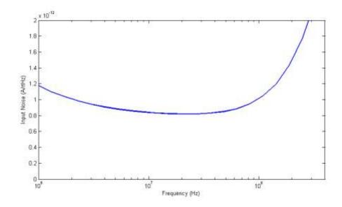
Fig. 26: Input referred noise at the TIA caused by the LPF.
