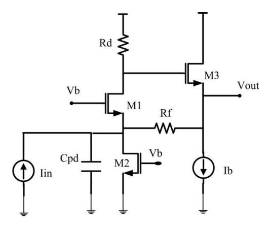
Fig. 6: Common gate architecture.
