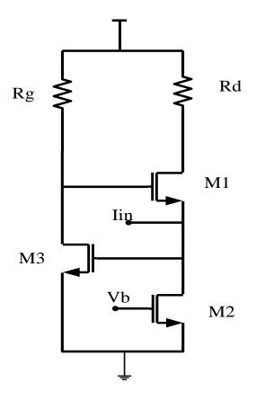
Fig. 8: Input of regulated gate cascode amplifier.
