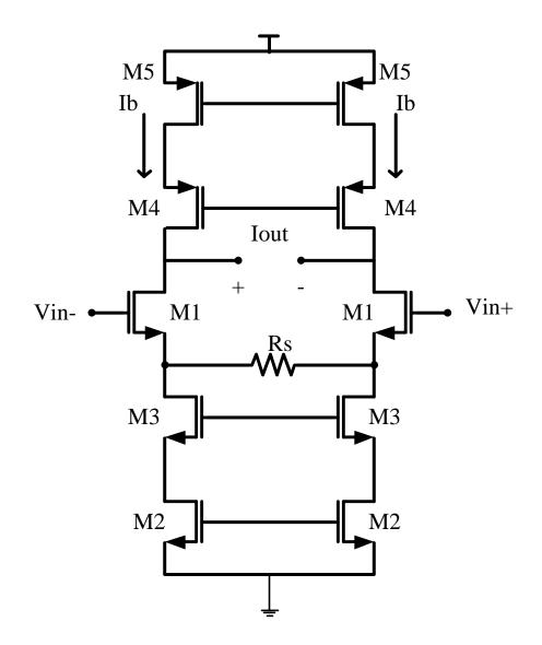
Fig. 20: Schematic of the transconductance amplifier used.
