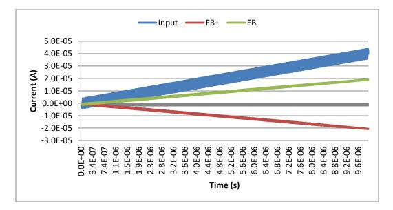
Fig. 36: Transient simulation showing input DC offest and feedback current
