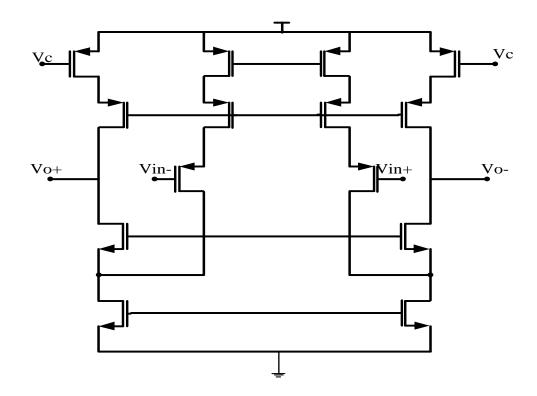
Fig. 19: Schematic of the amplifier used in the integrator.
