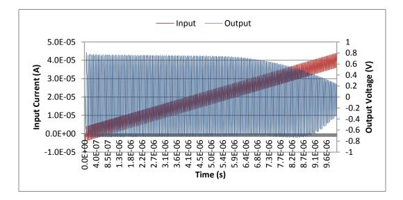
Fig. 35: Transient simulation with slow rising DC offset of 0A to 40µA.
