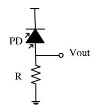
Fig. 3: Photodiode with load resistance.
