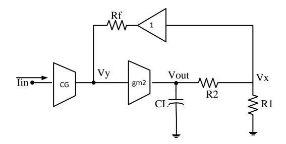
Fig. 13: A modified CH TIA with a common gate input stage.
