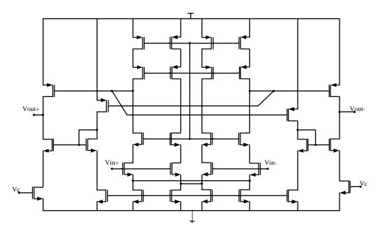
Fig. 18: Schematic of the opamp used in the LPF.
