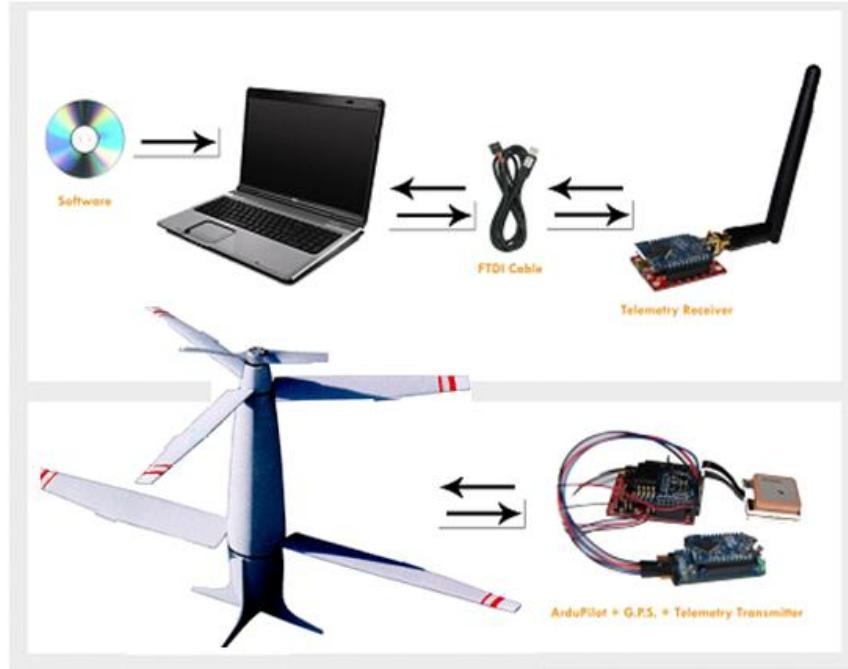
Figure 3.3. Ardupilot (Anderson, 2010) components and interface for Stop-Rotor UAV
