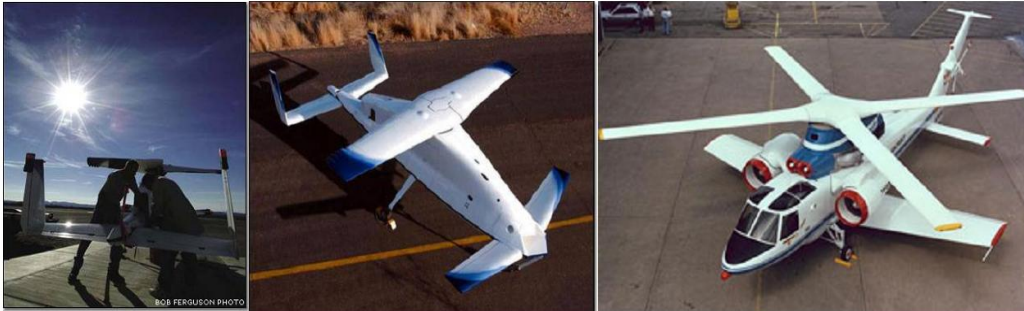
Figure 1.1. Stop-rotor aircrafts the X-50 Canard Rotor (left and middle) and Sikorsky X-Wing (right)
